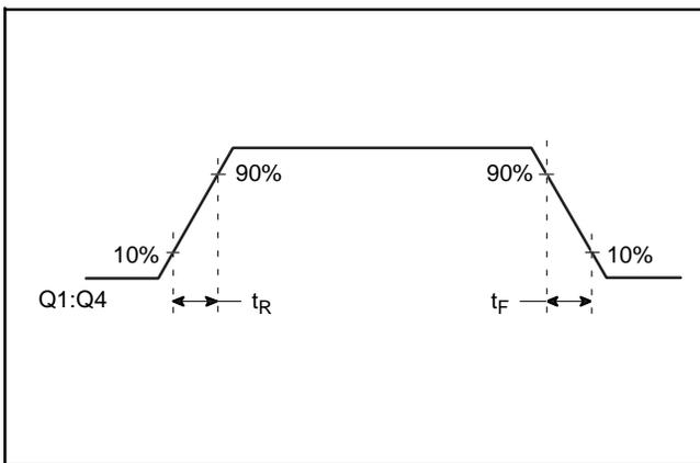
Figure 13. 2.5 V and 3.3 V Output Rise/Fall Time
