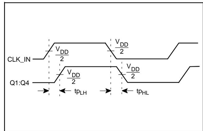
Figure 14. Propagation Delay
