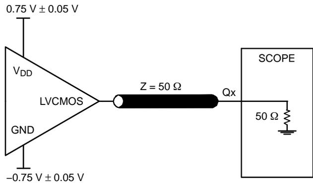
Figure 6. 1.5 V Output Load AC Test Circuit
