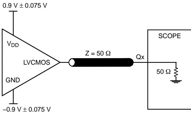
Figure 5. 1.8 V Output Load AC Test Circuit
