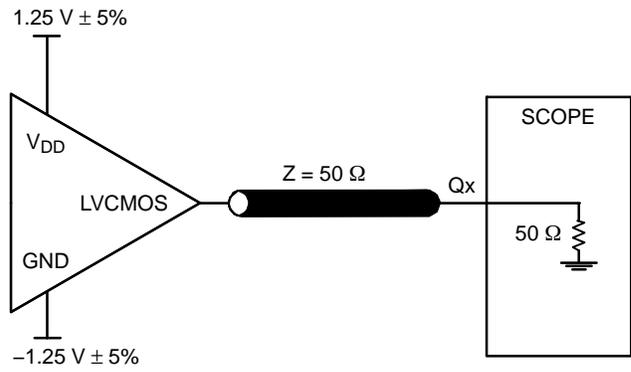
Figure 4. 2.5 V Output Load AC Test Circuit
