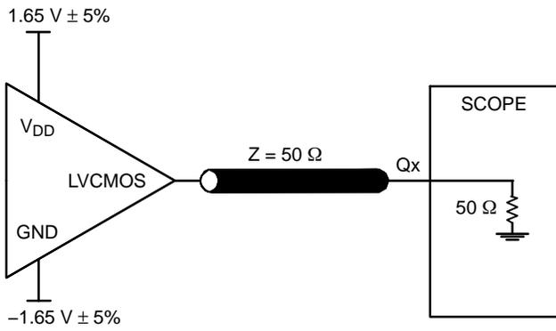
Figure 3. 3.3 V Output Load AC Test Circuit
