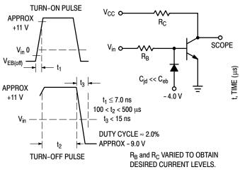
Figure 3. Switching Time Equivalent Circuit
