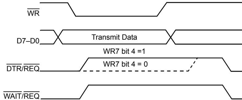
**Figure 12. DMA Request on Transmit Deactivation Timing**
