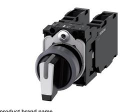
Selector switch, illuminable, 22 mm, round, plastic with metal front ring, white, selector switch, short, 3 switch positions I>O<II, momentary contact type, actuating angle 2x45°, 10:30h/12h/13:30h, with holder, 1 NO+1 NC, 1 NO+1 NC, screw terminal, with laser labeling, upper case
