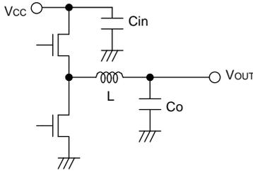
Figure.35 Input capacitor
