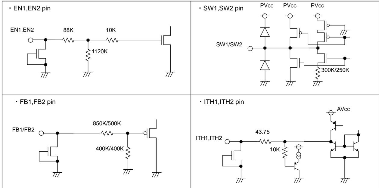
Figure.40 I/O equivalence circuit
