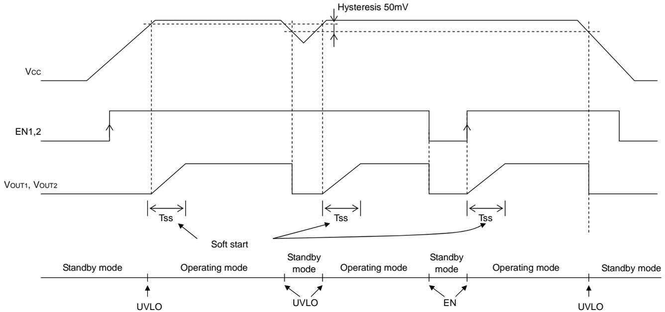
Figure.30 Soft start, Shut down, UVLO Timing chart
