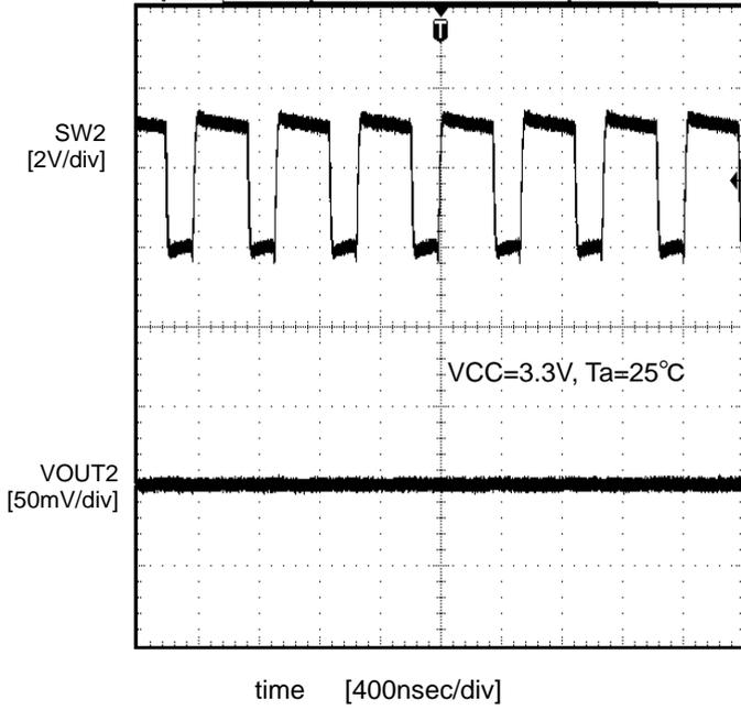
Figure.20 SW waveform 2
