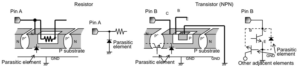
Figure.41 Simplified structure of monolithic IC
