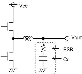
Figure.34 Output capacitor
