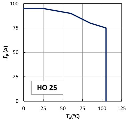
Figure 1:  $I_p$  vs  $T_A$  for HO series
