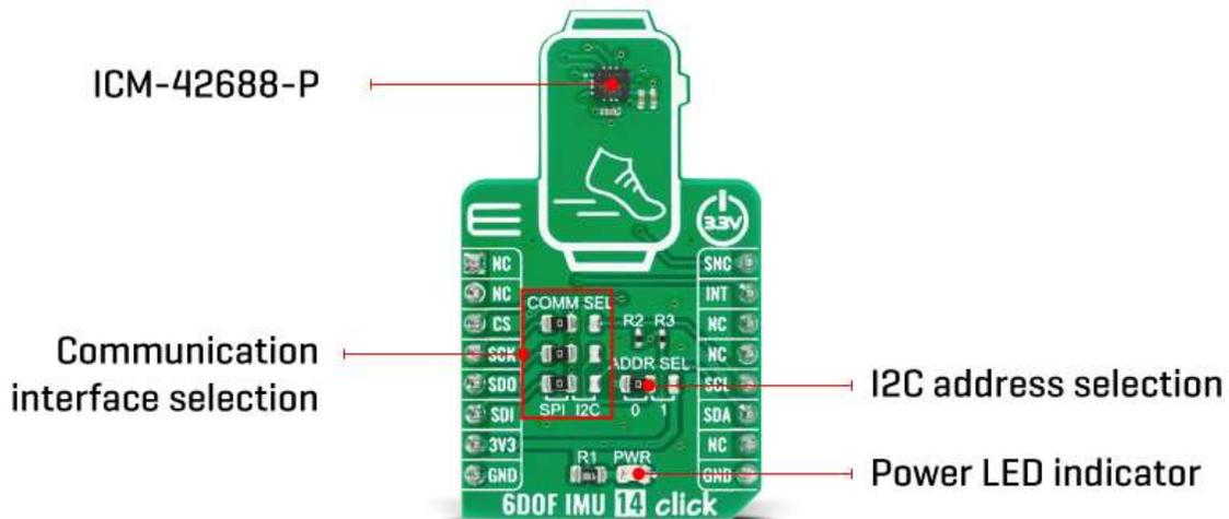
The ICM-42688-P architecture reduces the accelerometer's sensitivity to fabrication variations as well as to thermal drift. When the device is placed on a flat surface, it will measure 0g on the X- and Y-axes and +1g on the Z-axis. The full-scale range of the digital output can be adjusted from  $\pm 2g$ , up to  $\pm 16g$ .
