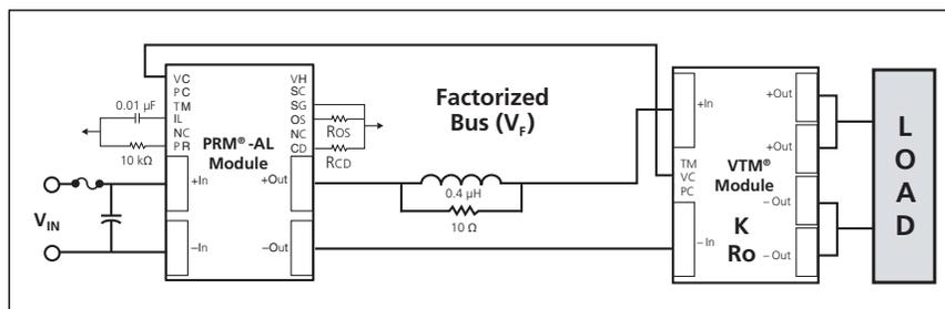
The P024F048T12AL is used with any 048 input series VTM to provide a regulated and isolated output.
