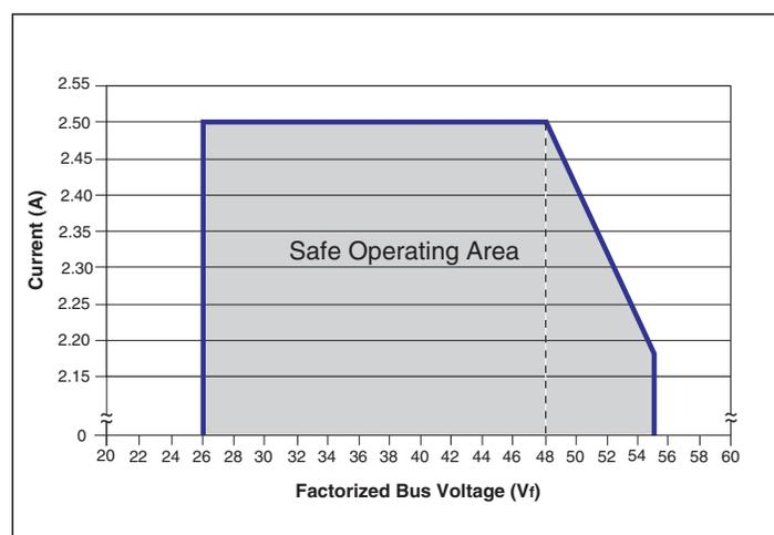
Figure 17 — P024F048T12AL rating based on Factorized Bus voltage
