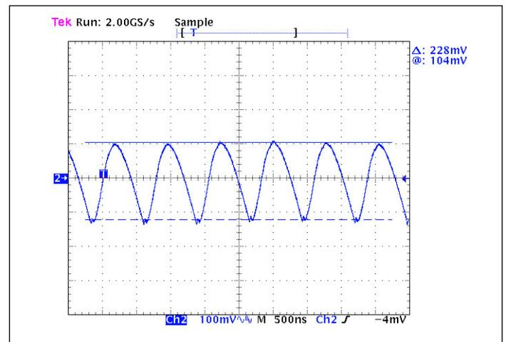
Figure 14 — Output ripple full load 10 µF bypass capacitance
