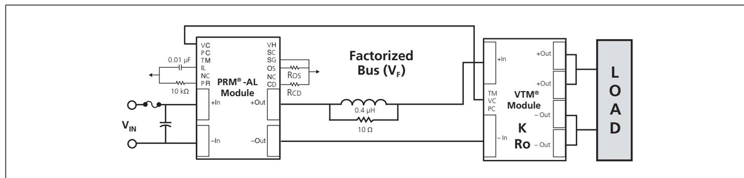
**Figure 1** — With Adaptive Loop control the output of the VTM is regulated over the load current range with only a single interconnect between the PRM and VTM and without the need for isolation in the feedback path.
