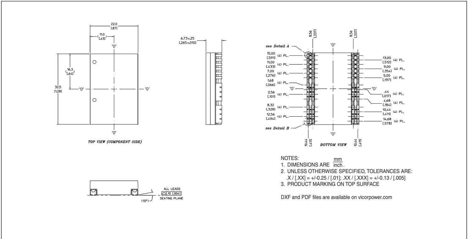
Figure 19 — PRM J-Lead mechanical outline; Onboard mounting
