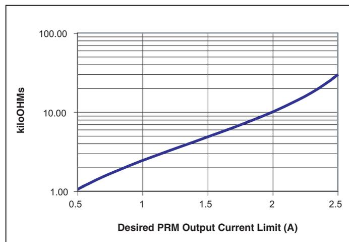
Figure 18 — External resistor value for adjusting current limit
