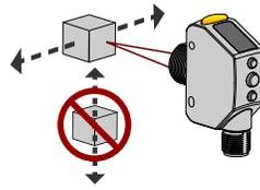
See the following figures for examples of correct and incorrect sensor-to-target orientation as certain placements may pose problems for sensing some targets. The Q4X can be used in the less preferred orientation and provide reliable detection performance; refer to the *Performance Curves* for the minimum object separation distance required for each case.
