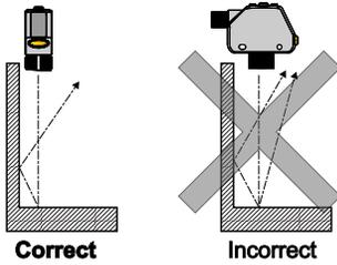
Figure 8. Orientation for a turning object
