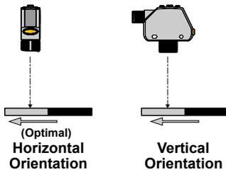
Figure 11. Orientation for highly reflective target<sup>¶</sup>
