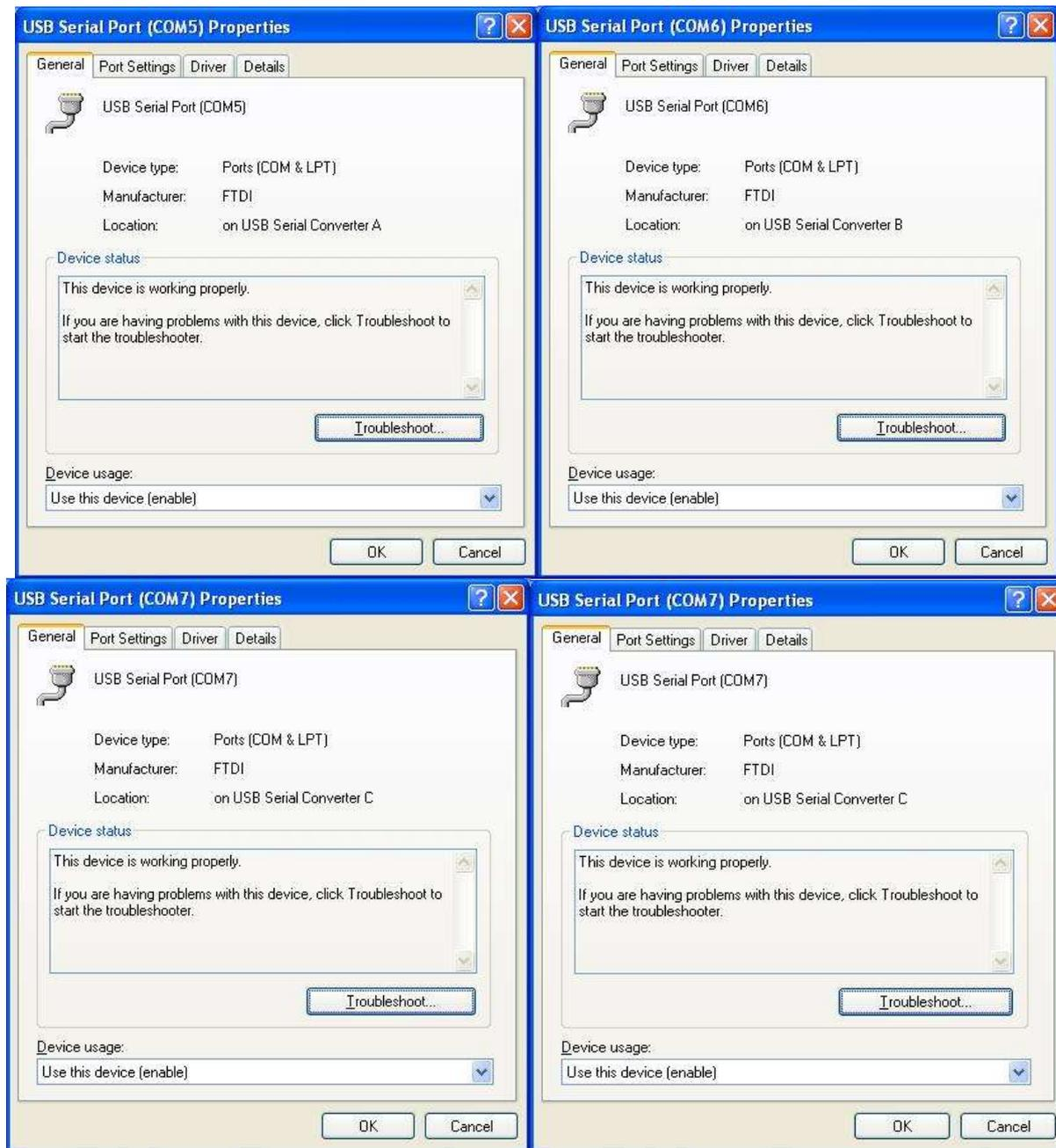
**Figure 2.12 – COM Port Assignment and Properties**
