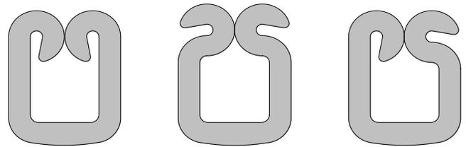
These crimp forms maybe changed completely by a small change in the wire, insulation punch, or terminal.
