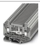
Test disconnect terminal block, Connection method: Screw connection, Cross section: 0.2 mm<sup>2</sup> -10 mm<sup>2</sup>, AWG: 24 - 8, Width: 8.2 mm, Mounting type: NS 35/7,5, NS 35/15, NS 32, Color: gray
