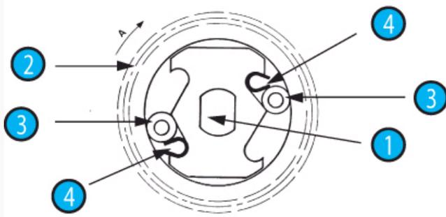
This device, situated inside the gearbox, enables the output shaft to be rotated by an external force (manual or mechanical) independently of the final wheel of the gearbox.
