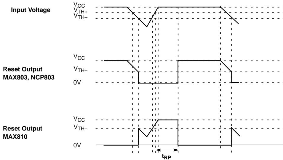
Figure 12. Timing Waveforms
