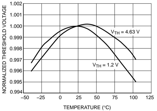
Figure 6. Normalized Reset Threshold Voltage vs. Temperature
