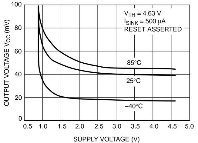
Figure 8. Output Voltage Low vs. Supply Voltage
