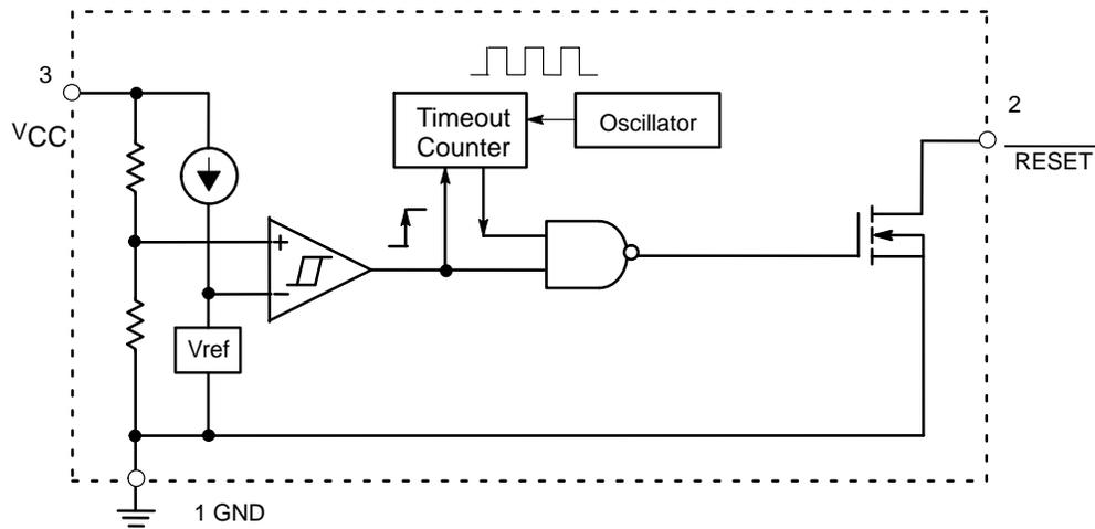
**Figure 2. NCP803, MAX803 Series Open-Drain Active-Low Output**
