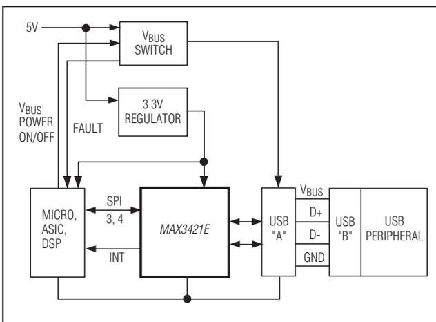
Figure 4. The MAX3421E in an Embedded Host Application
