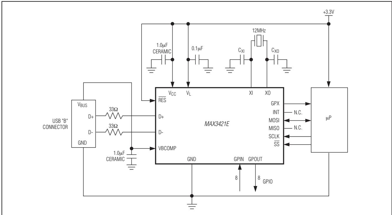
Figure 20. MAX3421E in a Self-Powered Peripheral Application
