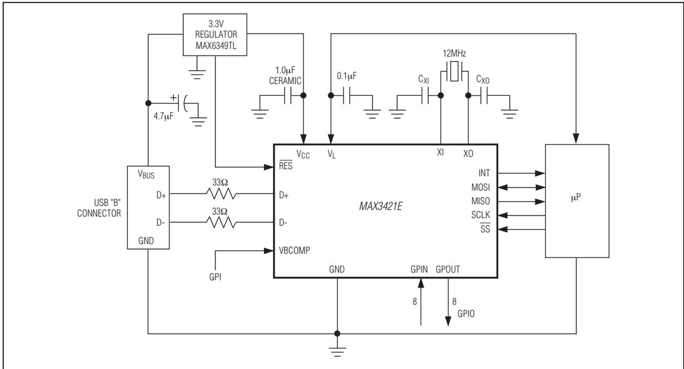
Figure 19. MAX3421E in a Bus-Powered Peripheral Application
