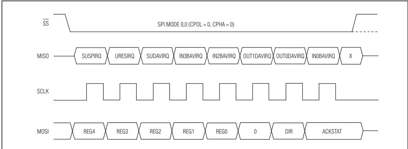
Figure 17. SPI Port in Full-Duplex Mode (Peripheral Mode)
