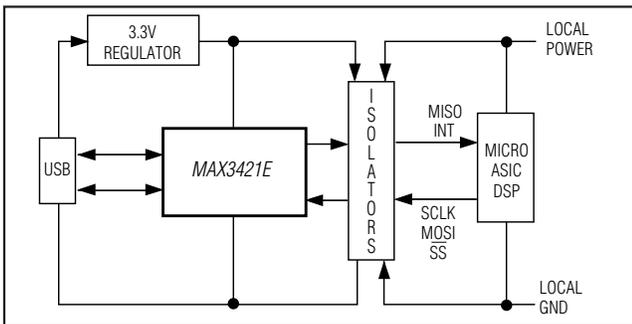
Figure 3. Optical Isolation of USB Using the MAX3421E
