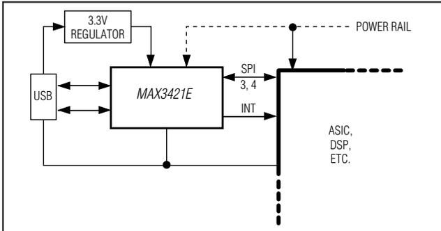
Figure 2. The MAX3421E Connected to a Large Chip
