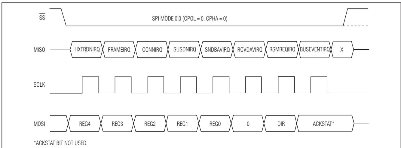
Figure 18. SPI Port in Full-Duplex Mode (Host Mode)
