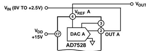
Figure 9. AD7528 in Single Supply, Voltage Switching Mode
