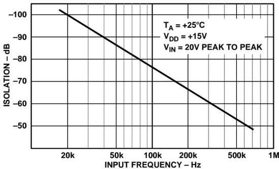
Figure 6. Channel-to-Channel Isolation
