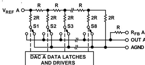
Figure 1. Simplified Functional Circuit for DAC A
