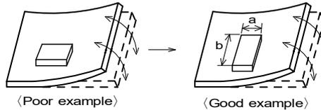
(2) Components location on PCB separation
