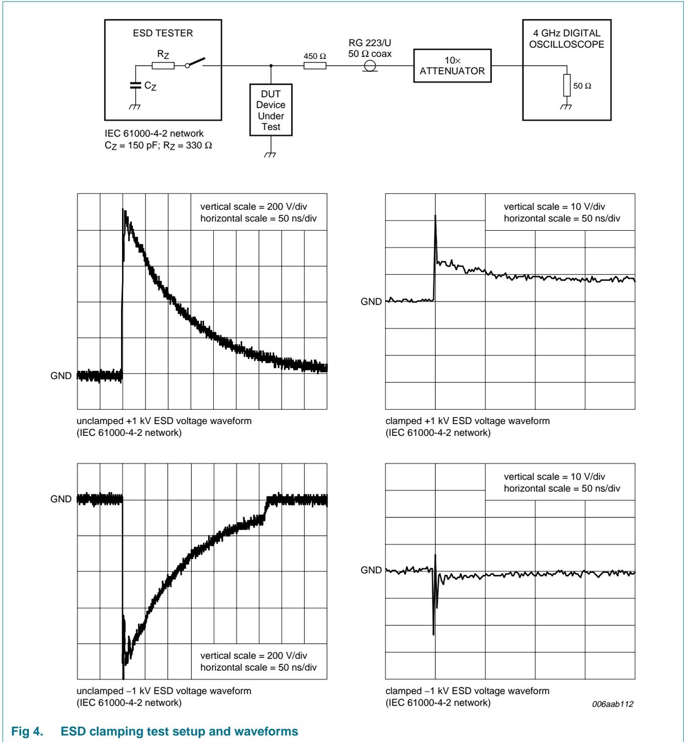
**Fig 4. ESD clamping test setup and waveforms**
