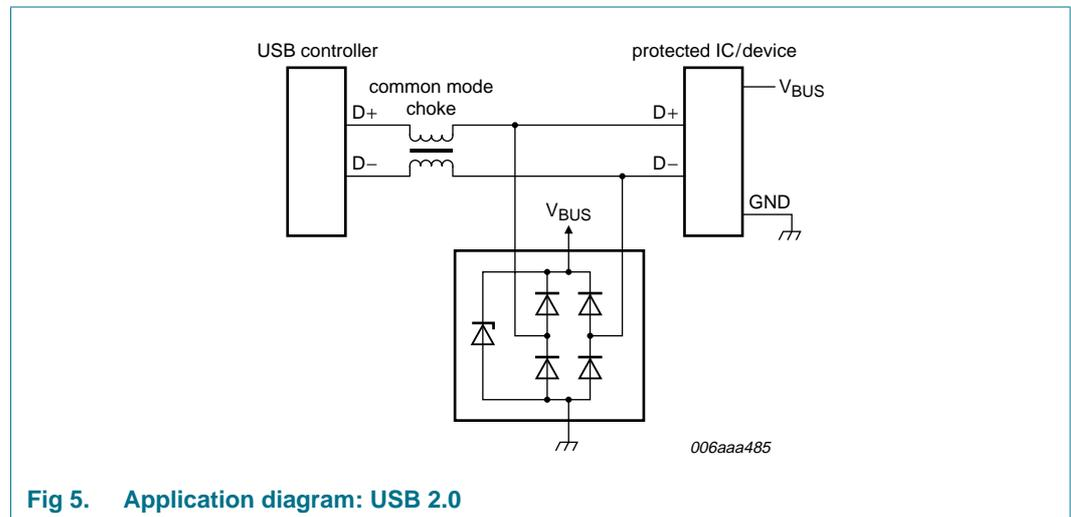
Fig 5. Application diagram: USB 2.0
