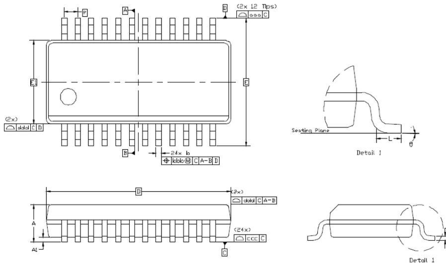
**Figure 6. 24-Pin SSOP**
