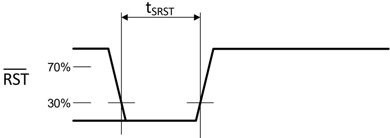
**Figure 1. Reset Timing**
