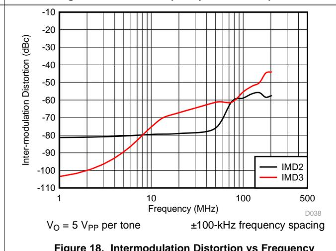
Figure 18. Intermodulation Distortion vs Frequency
