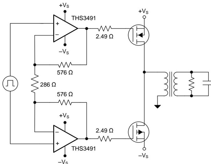
Figure 67. Power FET Drive Circuit
