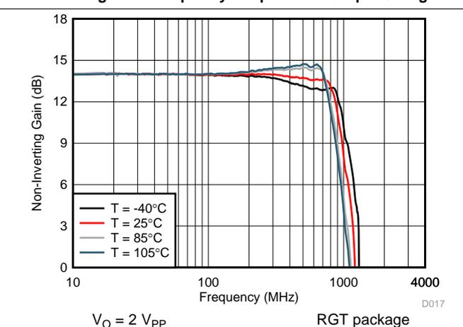
Figure 6. Frequency Response vs Temperature
