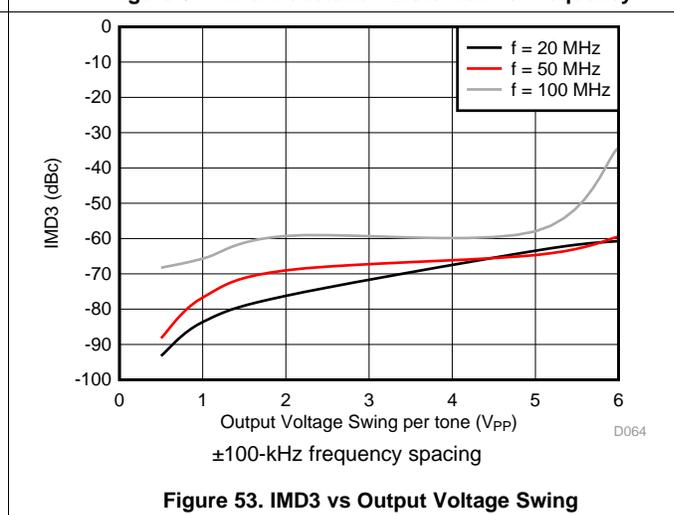
Figure 53. IMD3 vs Output Voltage Swing
