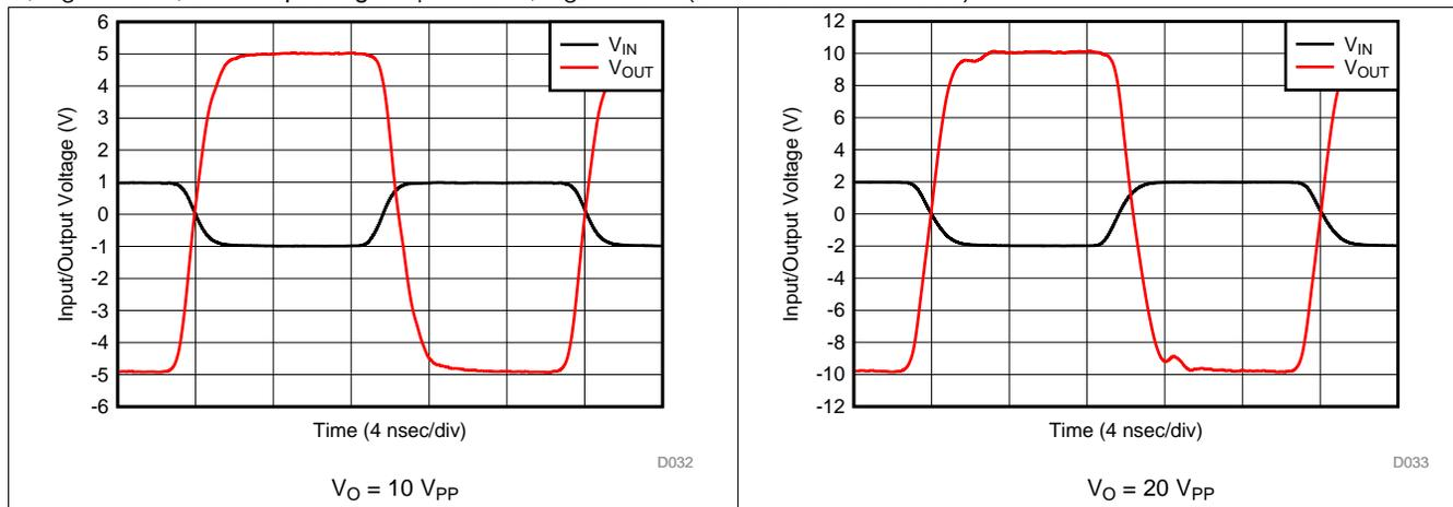
Figure 25.  $G = -5\text{ V/V}$  Pulse Response
