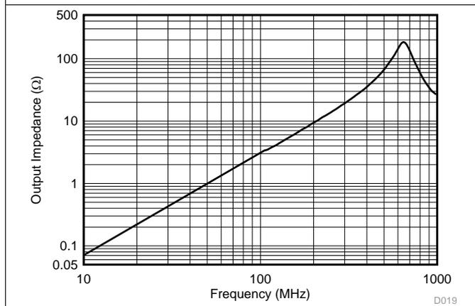
Figure 27. Output Impedance vs Frequency
