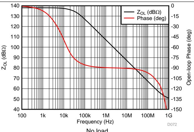
**Figure 22. Open-Loop Transimpedance Gain and Phase vs Frequency**
