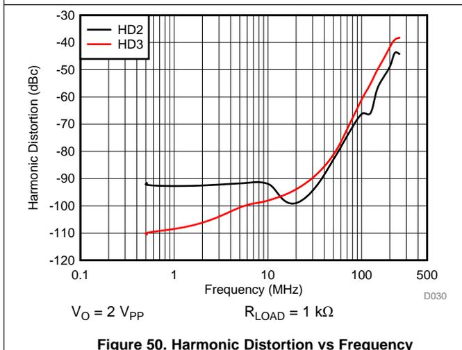
Figure 50. Harmonic Distortion vs Frequency
