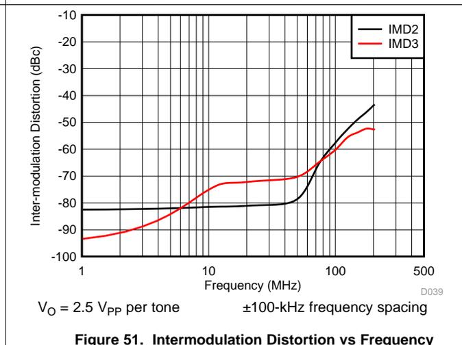
Figure 51. Intermodulation Distortion vs Frequency
