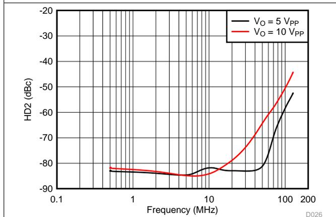
Figure 46. HD2 vs Frequency Across Output Swing
