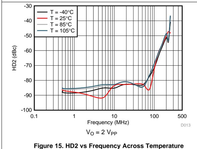
Figure 15. HD2 vs Frequency Across Temperature
