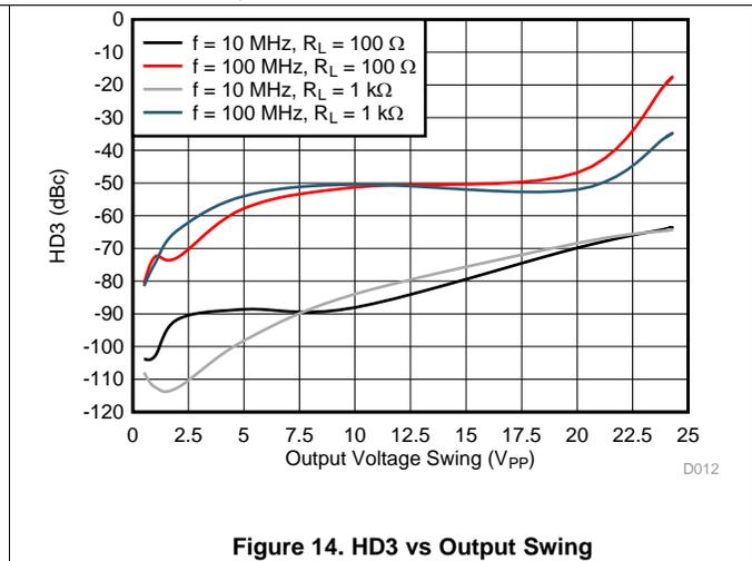
Figure 14. HD3 vs Output Swing
