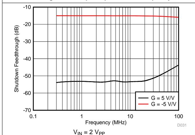
Figure 29. Shutdown Feedthrough vs Frequency
