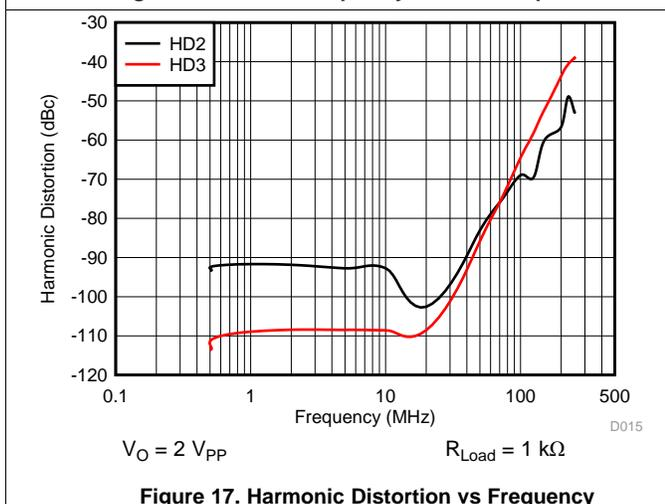
Figure 17. Harmonic Distortion vs Frequency
