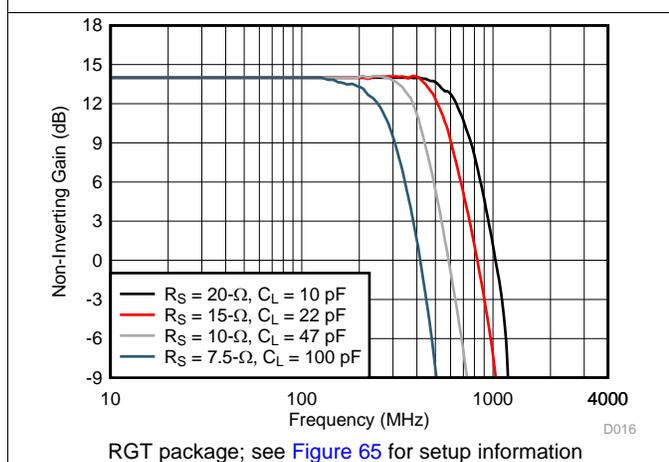
Figure 5. Frequency Response vs  $C_{LOAD}$
