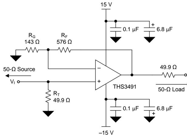
Figure 61. Wideband Noninverting Gain Configuration (5 V/V)
