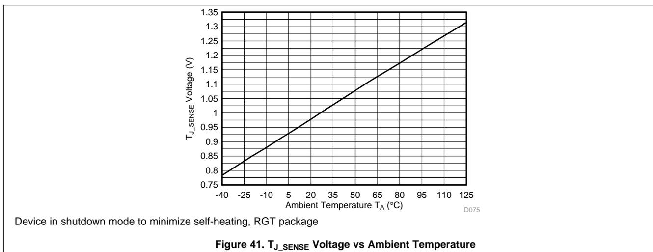
Figure 41.  $T_{J\_SENSE}$  Voltage vs Ambient Temperature
