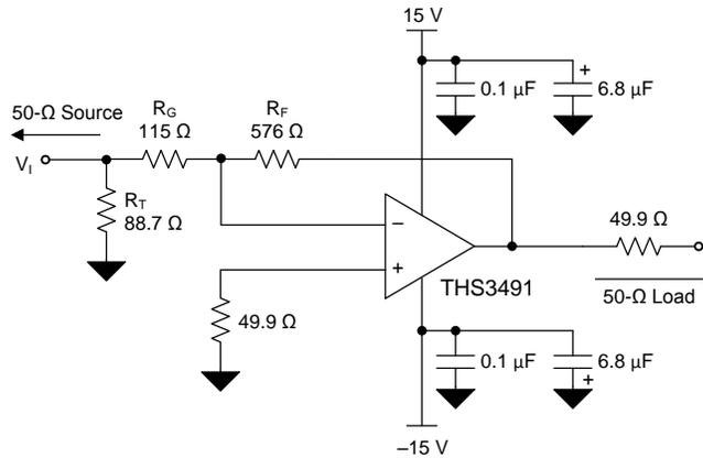
Figure 62. Wideband Inverting Gain Configuration (5 V/V)
