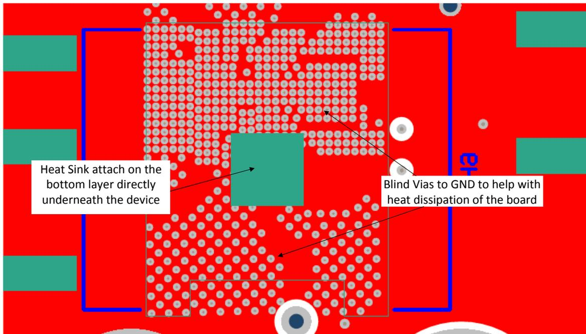
Figure 78. Heat Sink Attachment to Bottom Layer
