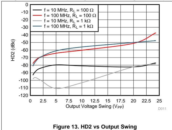
Figure 13. HD2 vs Output Swing
