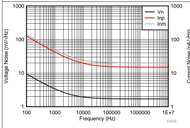
**Figure 21. Spot Input Noise vs Frequency**
