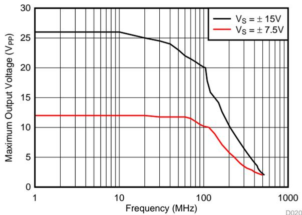
**Figure 64. Maximum Recommended Output Voltage vs Frequency**
