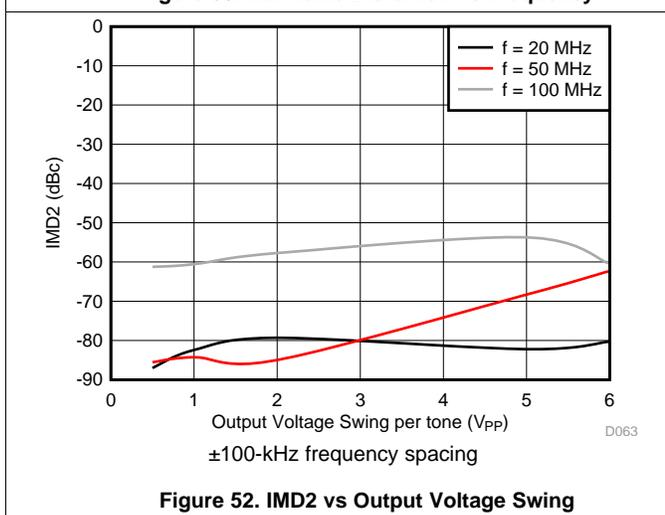
Figure 52. IMD2 vs Output Voltage Swing
