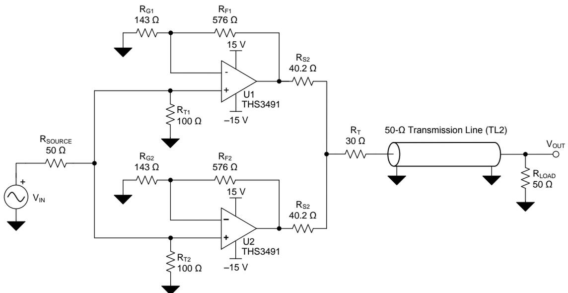
Figure 69. Load-Sharing Driver Application
