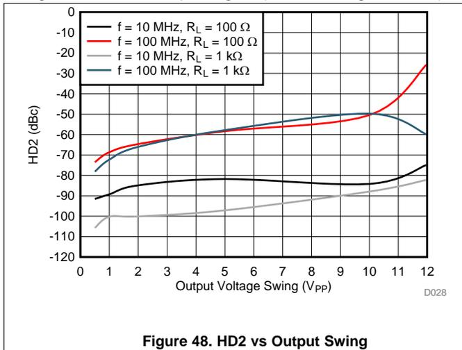
Figure 48. HD2 vs Output Swing
