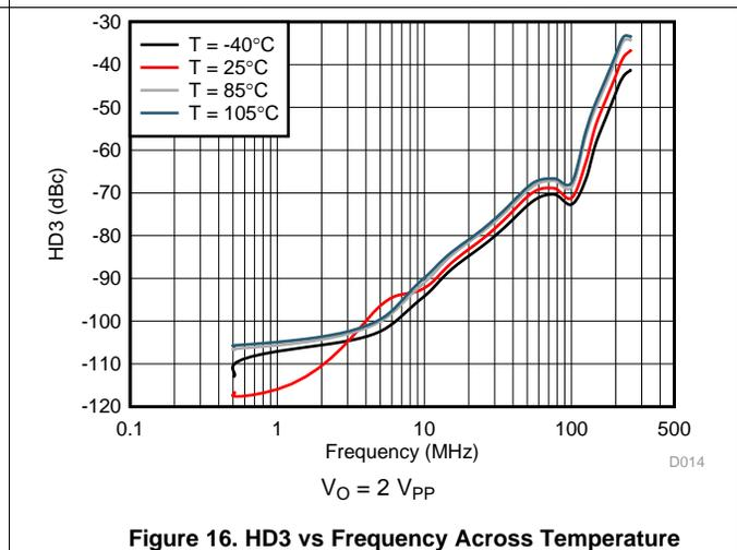
Figure 16. HD3 vs Frequency Across Temperature
