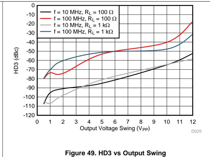
Figure 49. HD3 vs Output Swing
