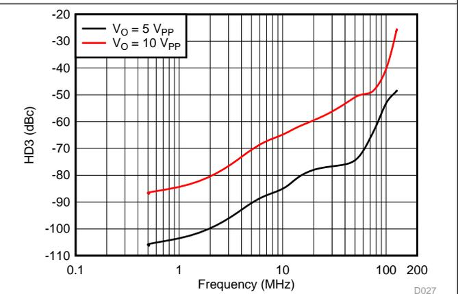
Figure 47. HD3 vs Frequency Across Output Swing
