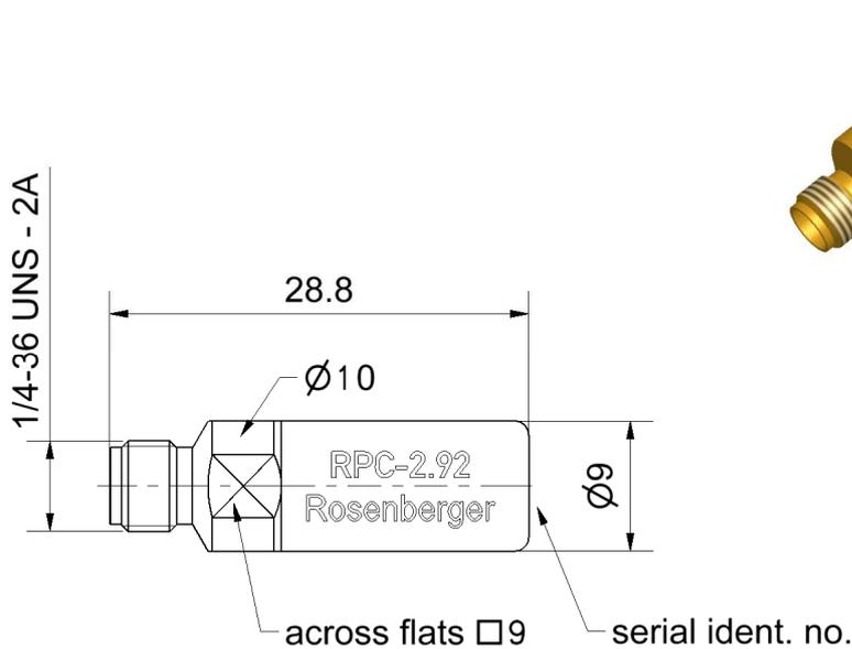
All dimensions are in mm; tolerances according to ISO 2768 m-H
