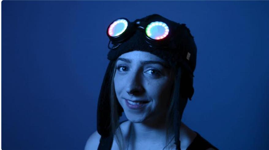
Adafruit NeoPixel LED rings fit perfectly inside the eyecups of most 50mm round goggles — a very common size. It's almost as if these rings were made with this project in mind!
