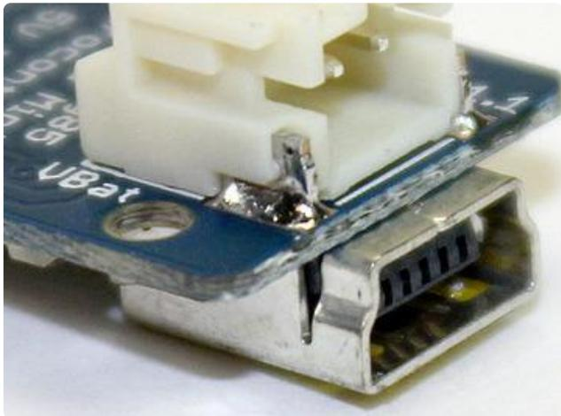
Hold the JST socket in place (tweezers recommended) and re-melt the solder, allowing the part to sink into position.
