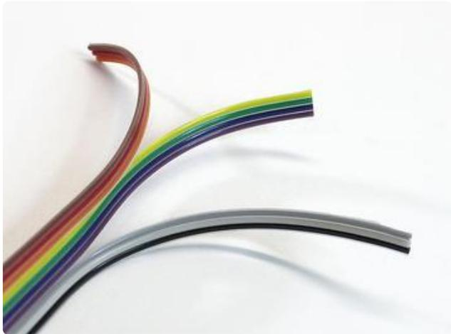
Next, peel away two sets of three wires each from the included bit of ribbon cable. (If you're building your own custom goggles, you can just use separate pieces of wire for this, it's all good.)
