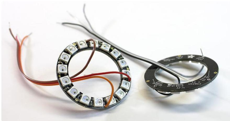
Notice how the wires are inserted from the front, then soldered on the back of the ring. Do it this way if you're new to soldering...it's much easier. It can work the other way too...insert from back, solder on front...but the component tolerances are extremely tight and beginners often get a blob of solder in the wrong place and the LEDs don't work.
