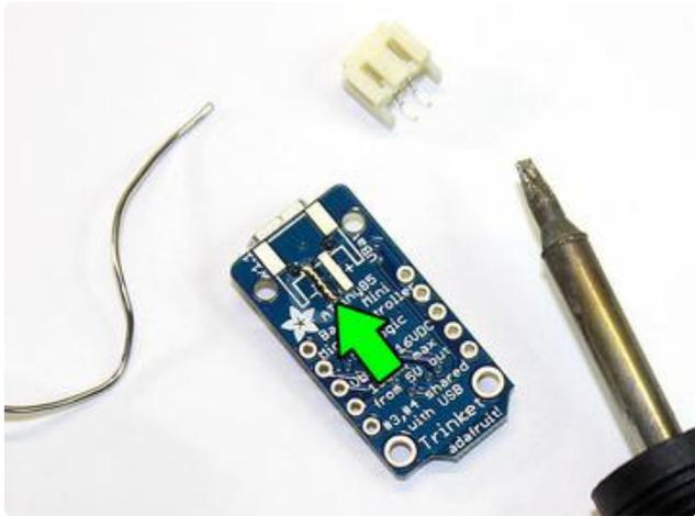
Start by “tinning” one of the JST pads on the back of the Trinket...heat the pad and apply solder so the whole surface is coated.
