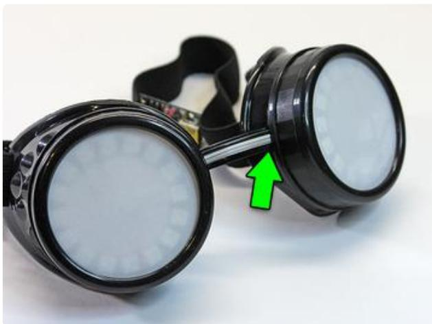
Screw the lenses in place, being super extra careful not to gouge the wires!
