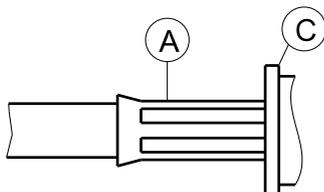
Slide ferrule A over braid and crimp as close to connector body C as possible.
