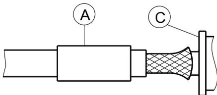
Splay out braid and insert cable in connector body C until contact B engages perceptibly. Ensure that braid lies above the crimp neck.
