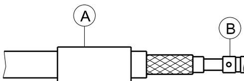
Push contact B over inner conductor to abut cable dielectric and crimp.
