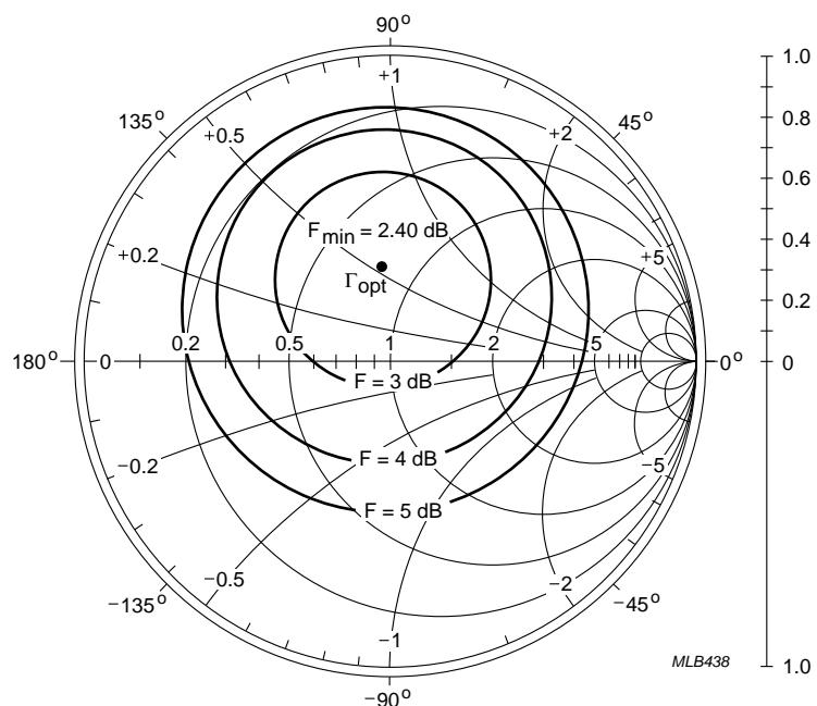
$V_{CE} = -5 \text{ V}$ ;  $I_C = -10 \text{ mA}$ ;  $f = 500 \text{ MHz}$ ;  $Z_0 = 50 \Omega$ .
