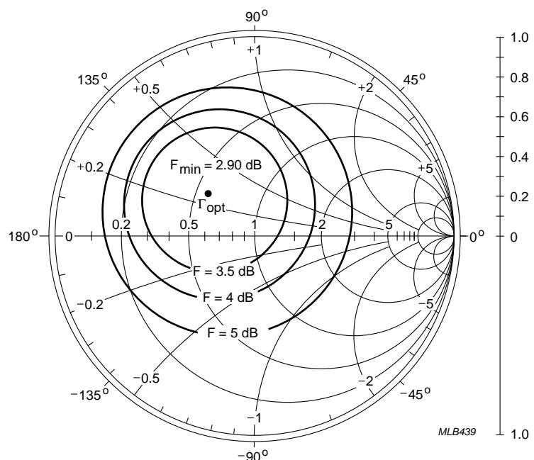
$V_{CE} = -5 \text{ V}$ ;  $I_C = -10 \text{ mA}$ ;  $f = 1 \text{ GHz}$ ;  $Z_0 = 50 \Omega$ .
