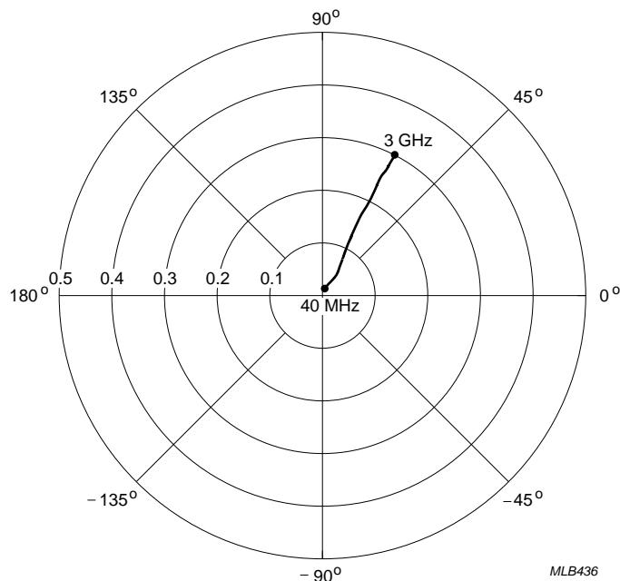
$V_{CE} = -10 \text{ V}; I_C = -30 \text{ mA.}$ Fig.12 Common emitter reverse transmission coefficient ( $s_{12}$ ), typical values.
