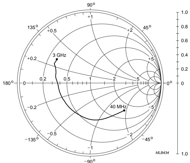
$V_{CE} = -10 \text{ V}; I_C = -30 \text{ mA}.$ Fig.10 Common emitter input reflection coefficient ( $s_{11}$ ), typical values.
