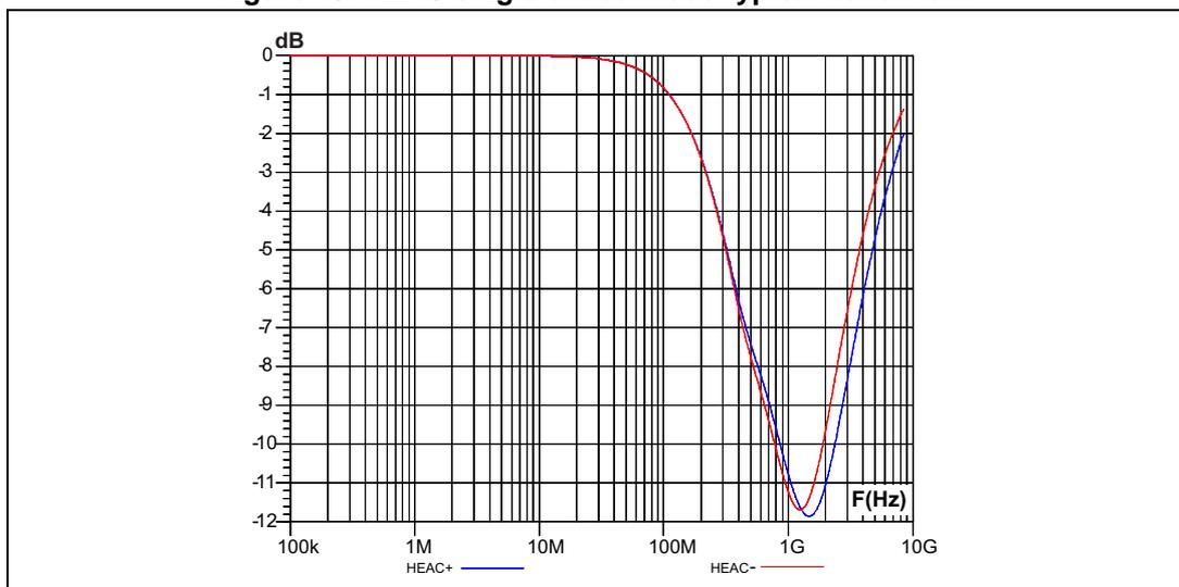
Figure 19. TMDS line S<sub>21</sub> frequency response
