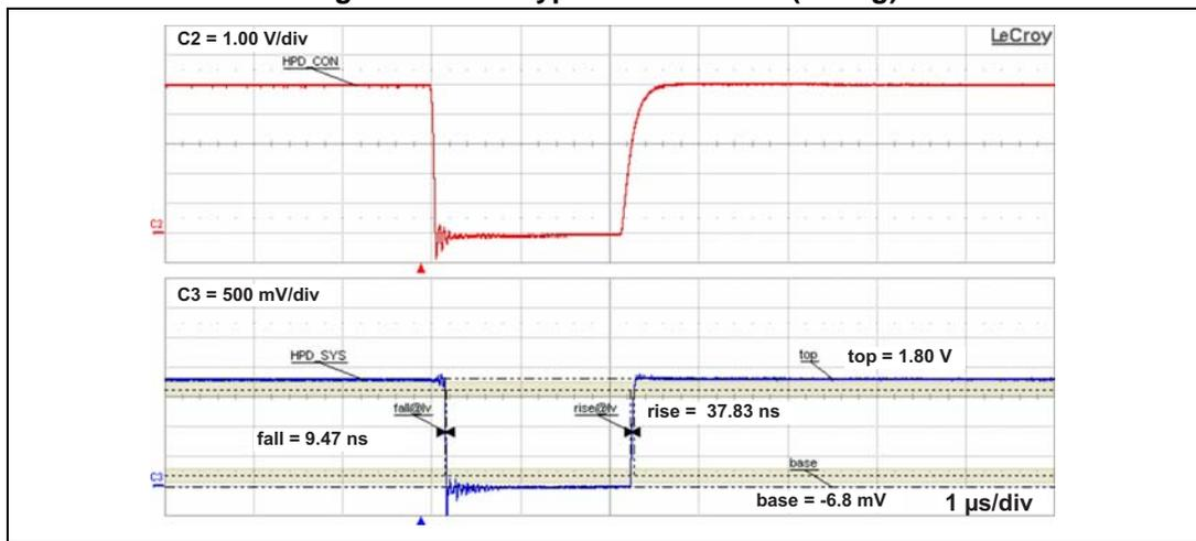
Figure 18. HEAC single ended mode typical bandwidth
