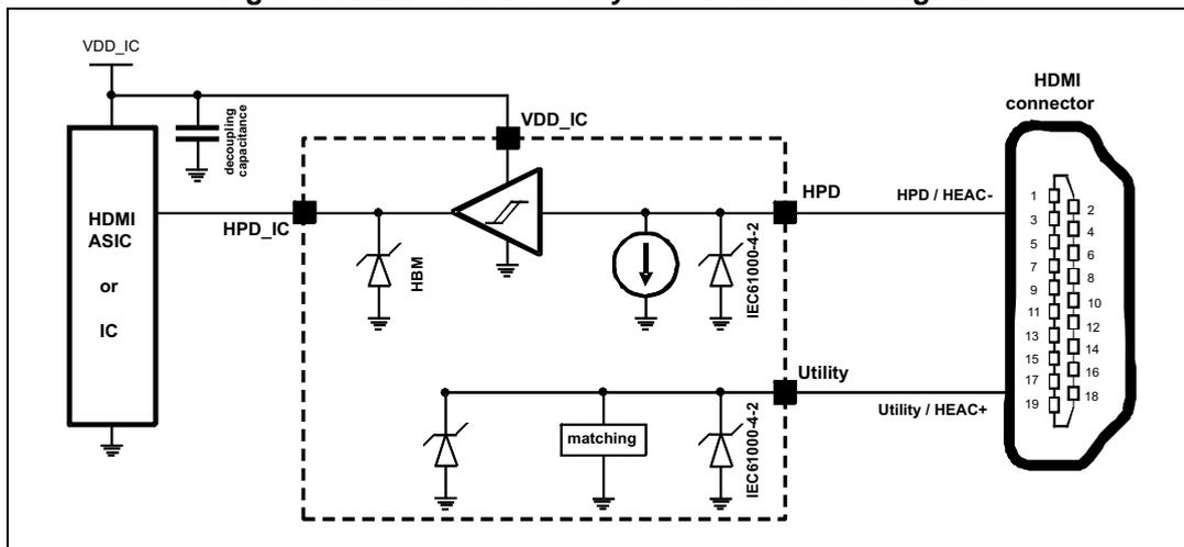
This block simplifies the design and the PCB layout of the HPD and HEAC functions.
