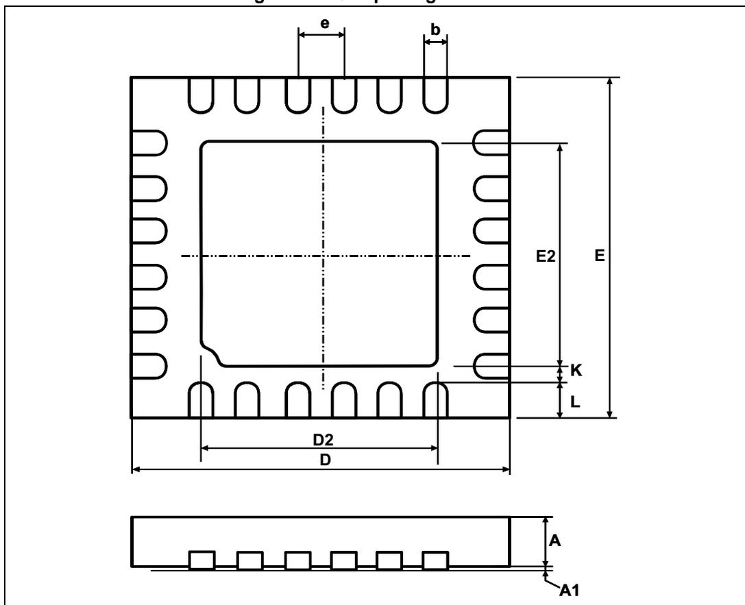
Table 10. QFN package mechanical data
