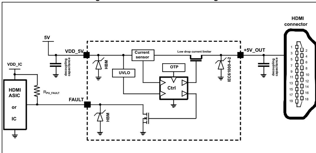
To summarize, the short circuit protection and the over temperature protection features are providing a high robustness level of the application. On top of this, the fault line feature can be used in order to improve the user experience.
