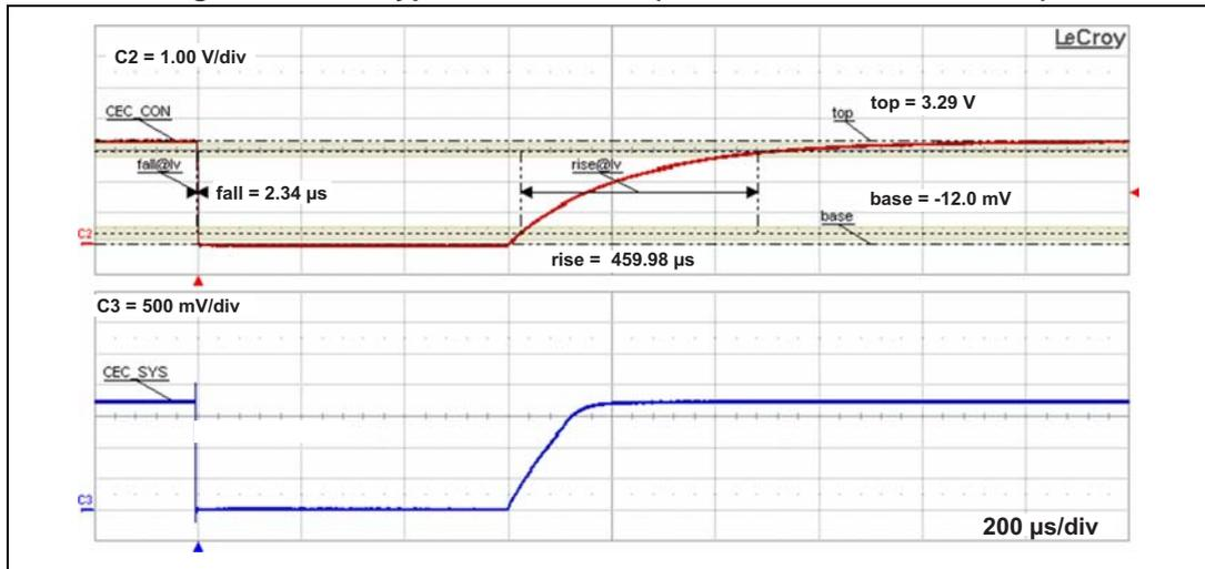
Figure 14. CEC typical waveforms (cable to IC communication)
