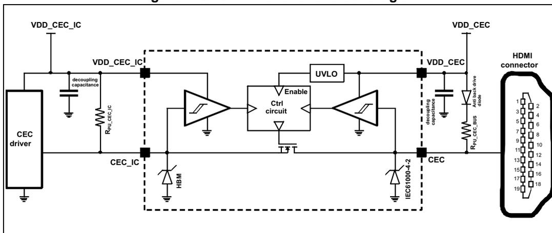
In case of no activity on the CEC bus, or if the CEC driver is off ( $V_{DD\_CEC} = 0$ ), the output CEC pin is put in high impedance mode (open circuit) protecting the circuitry and the application against hazardous backdrive.
