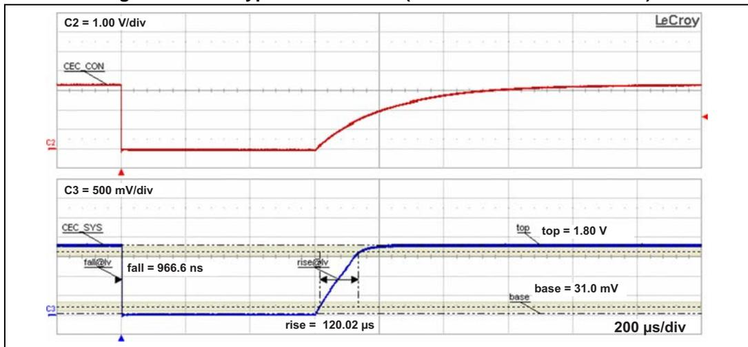
Figure 15. DDC typical waveforms (IC to cable communication)
