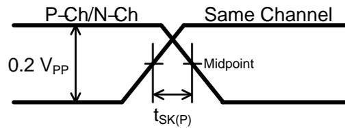
Figure 8.  $t_{SK(P)}$ , Same Channel Opposite Transitions
