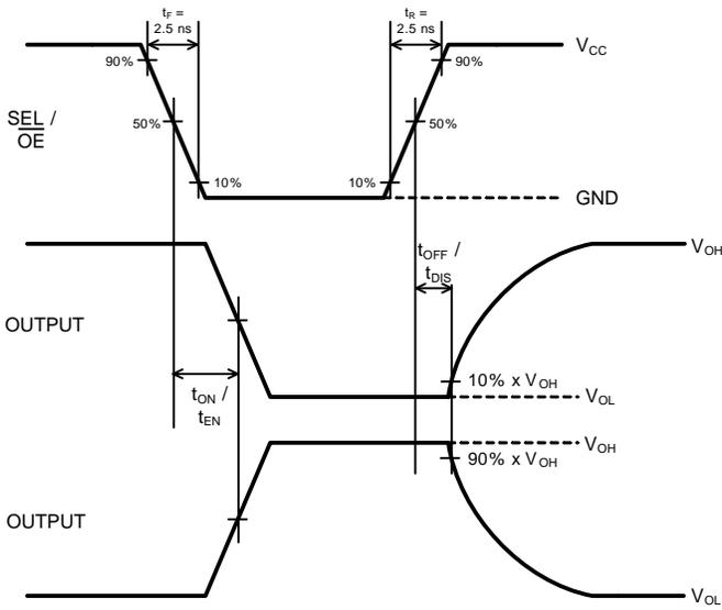
Figure 5.  $t_{EN}$ ,  $t_{DIS}$ ,  $t_{ON}$ ,  $t_{OFF}$  Times
