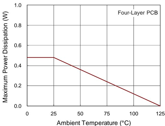
Figure 3. Derating Curves of Maximum Power Dissipation
