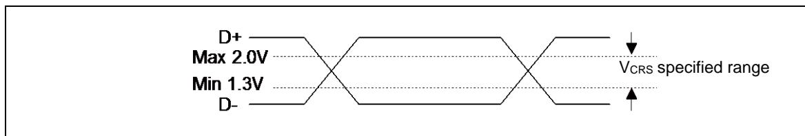
\*5: They indicate rise time ( $t_{RISE}$ ) and fall time ( $t_{FALL}$ ) of the full-speed differential data signal.
