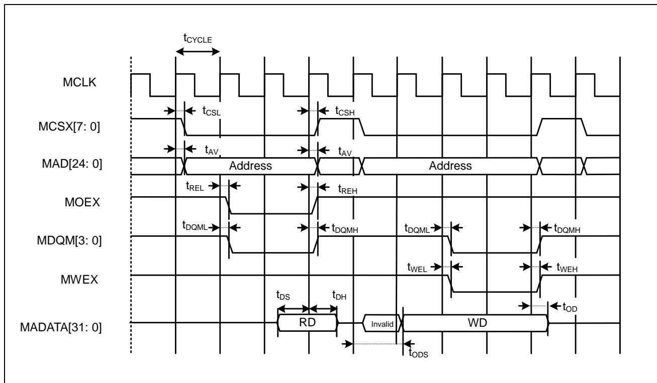
**Multiplexed Bus Access Asynchronous SRAM Mode**
