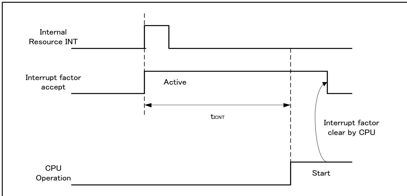
\*: Depending on the standby mode, interrupt from the internal resource is not included in the recovery cause.
