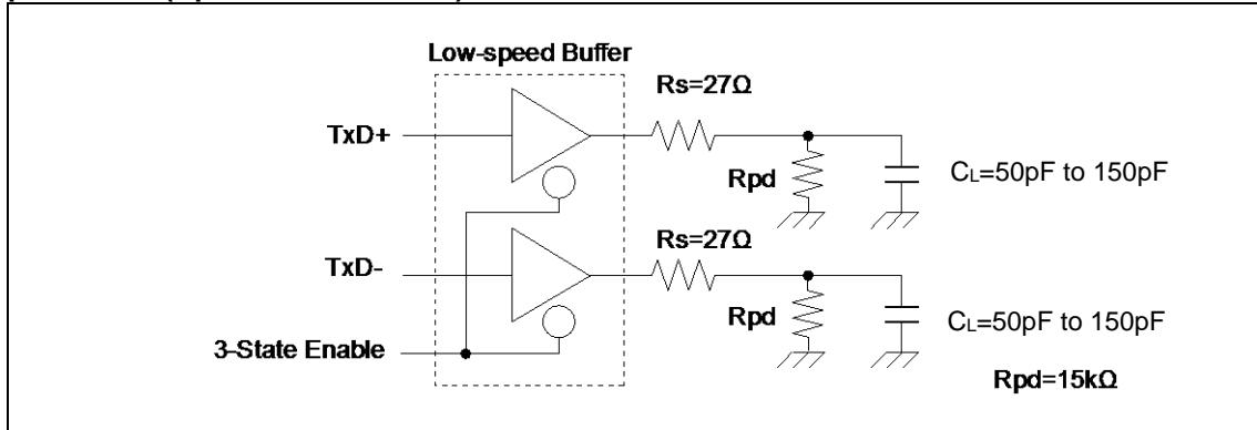
**Low-Speed Load (Downstream Port Load) - Reference 2**
