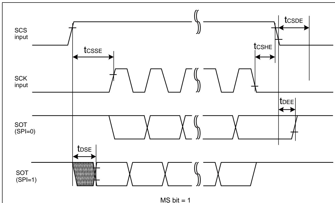
**High-Speed Synchronous Serial (SPI = 0, SCINV = 0)**
