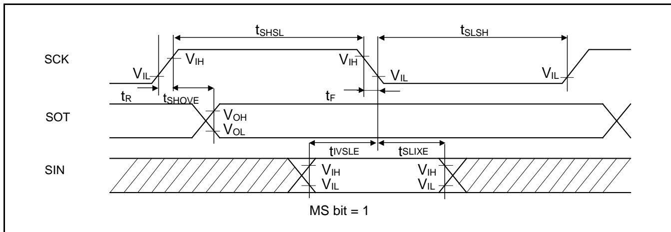
**Synchronous Serial (SPI = 1, SCINV = 0)**
