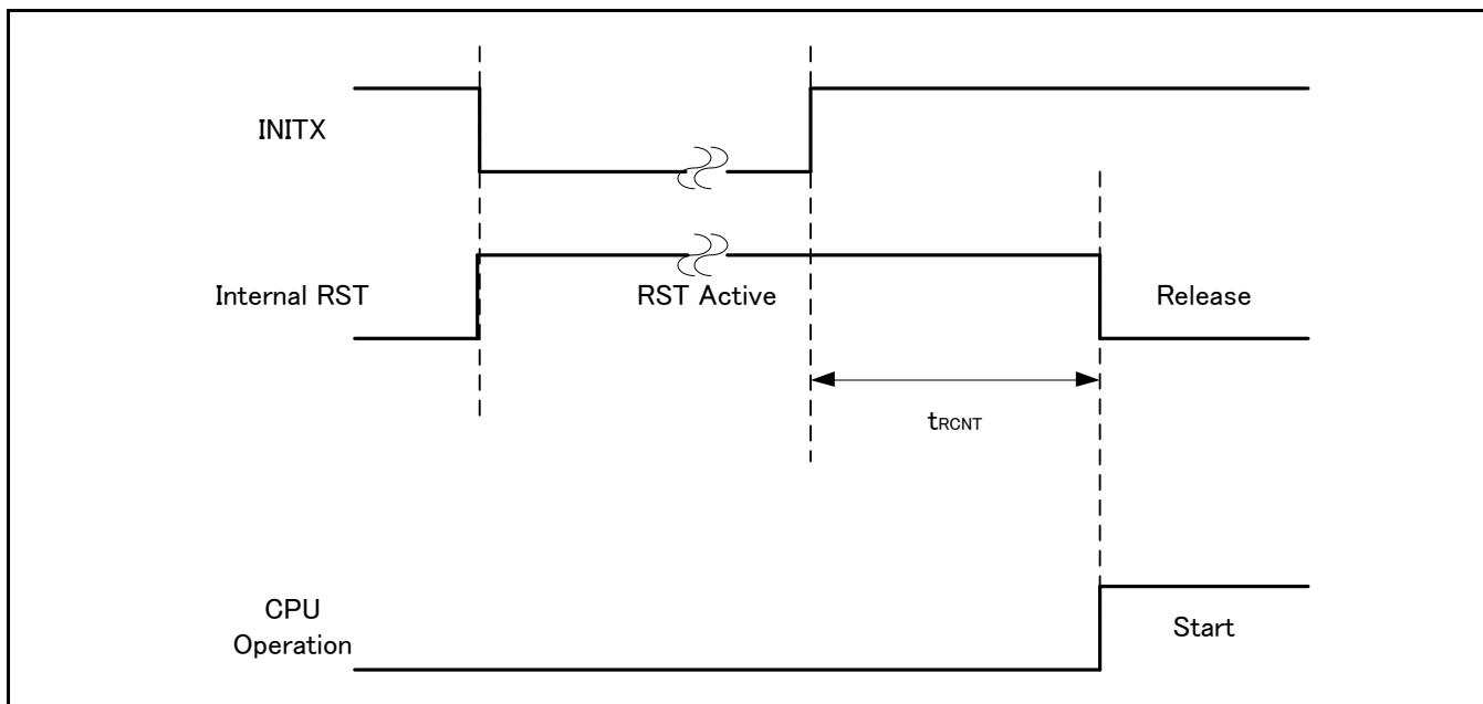
**Example of Standby Recovery Operation (when in Internal Resource Reset Recovery\*)**
