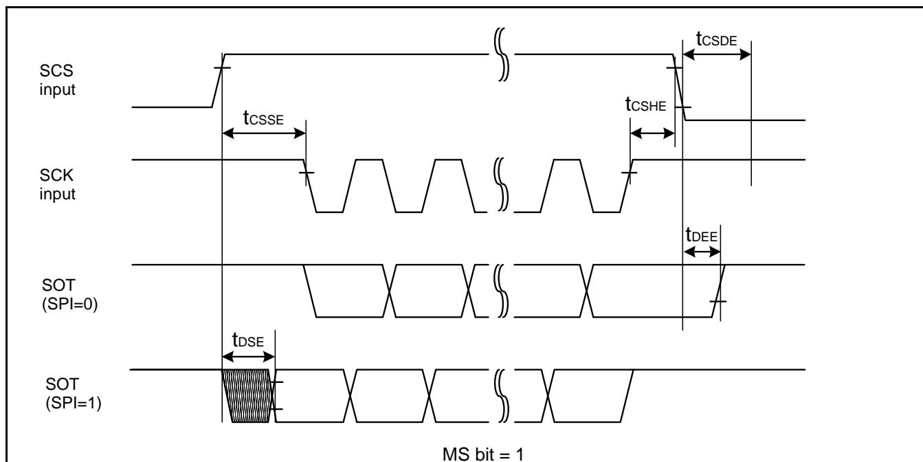
**When Using High-Speed Synchronous Serial Chip Select (SCINV = 1, CSLVL = 0)**
