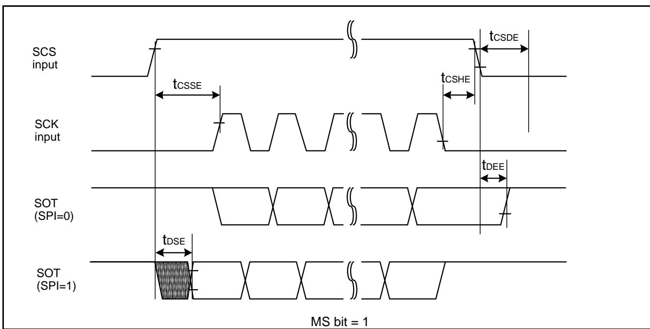
**External Clock (EXT = 1): When in Asynchronous Mode Only**
