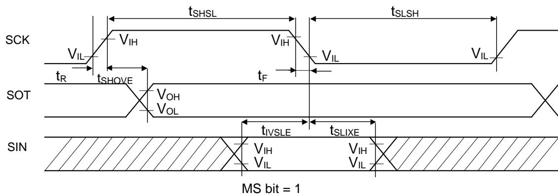
**High-Speed Synchronous Serial (SPI = 1, SCINV = 0)**
