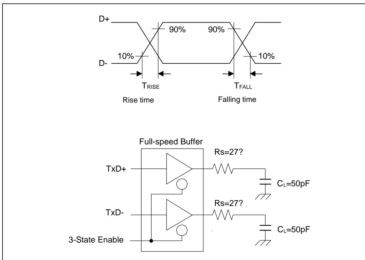
\*6: USB Full-speed connection is performed via twisted-pair cable shield with  $90\Omega \pm 15\%$  characteristic impedance (differential mode).
