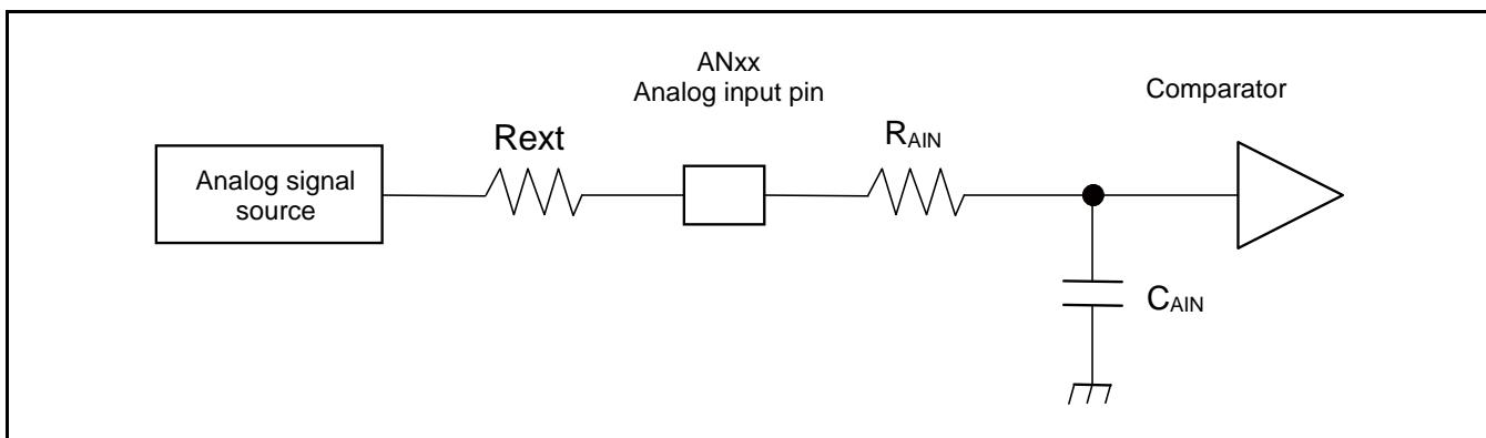
(Equation 1)  $t_s \geq (R_{AIN} + R_{ext}) \times C_{AIN} \times 9$
