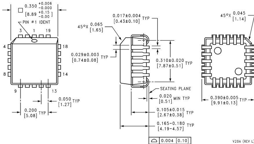
**Molded Chip Carrier Package (V)**
