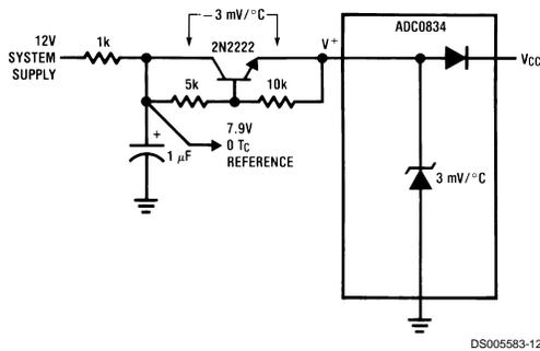
FIGURE 4. Operating with a Temperature Compensated Reference
