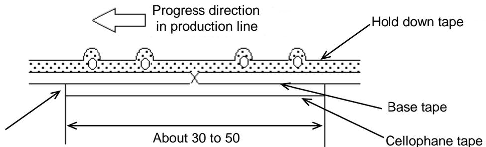
No lifting for the direction of progressing
