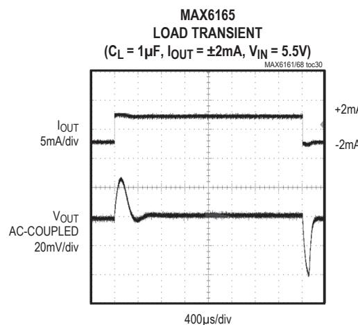
**Typical Operating Characteristics (continued)**(V<sub>IN</sub> = +5V for MAX6161–MAX6168, V<sub>IN</sub> = +5.5V for MAX6165, I<sub>OUT</sub> = 0, T<sub>A</sub> = +25°C, unless otherwise noted.) (Note 5)
