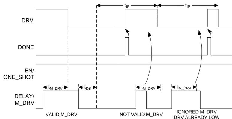
Figure 11. Manual MOSFET Power ON in Timer Mode
