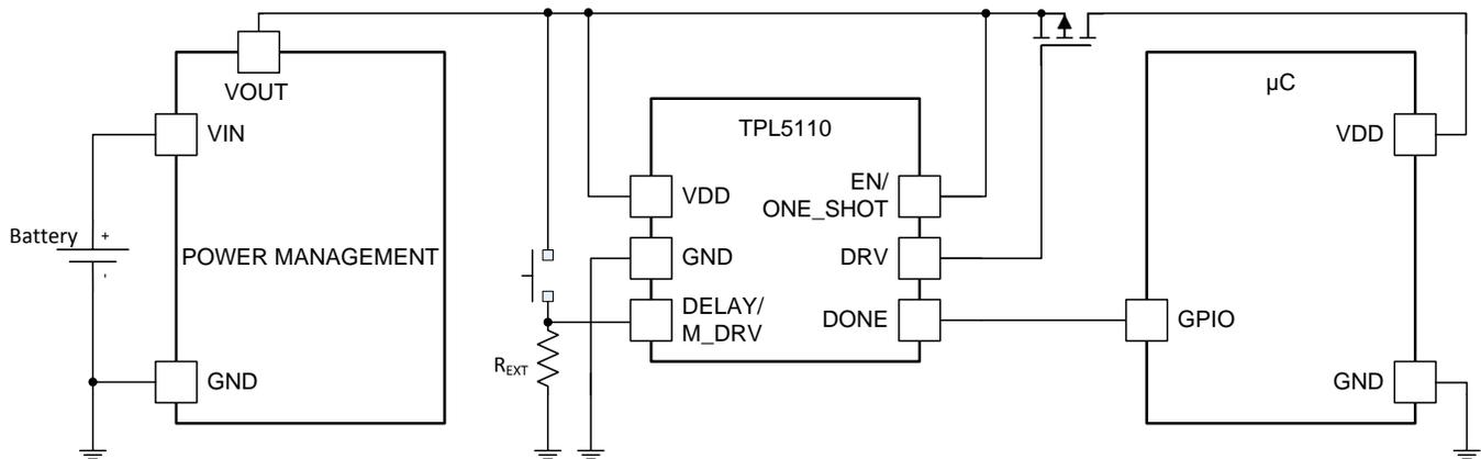
**Figure 13. Manual MOSFET Power ON With SPST Switch**
