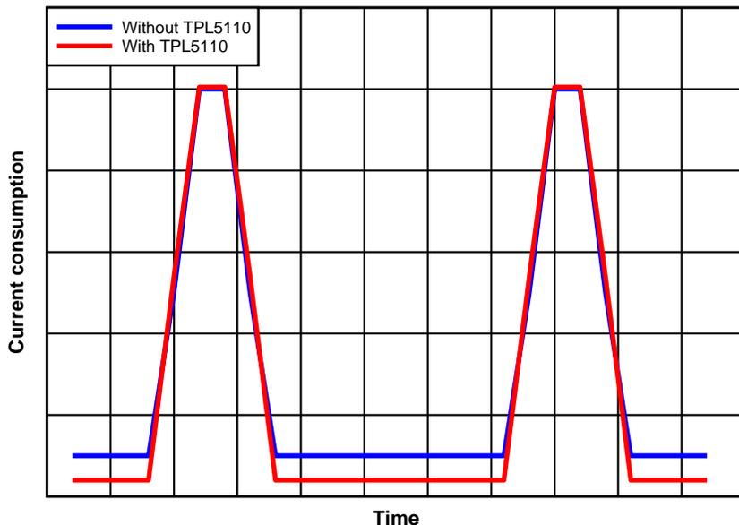
Figure 16. Effect of TPL5110 on Current Consumption
