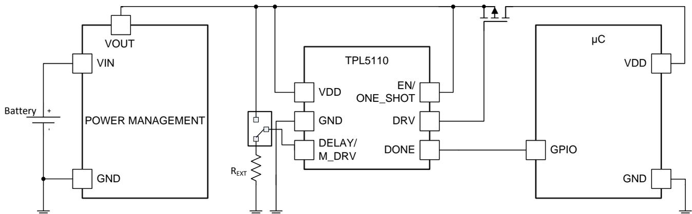
**Figure 14. Manual MOSFET Power ON With SPDT Switch**
