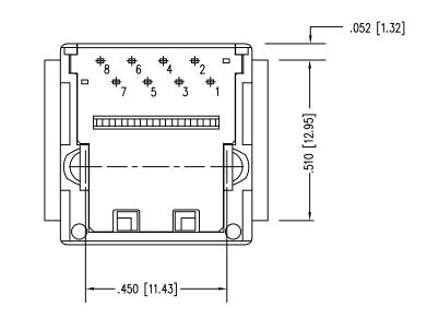
.050 [1.27] -TYP. .100 [2.54] .050 [1.27]ø.035 [0.89] ±.003 [0.08] (8) ф Ø.006 [0.15] ø .125 [3.18] .128 [3.25] (2) - .450 [11.43] ф Ø.006 [0.15]
