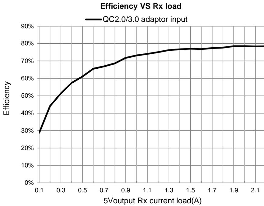
Note: Both results are measured with TSDMRX-5V/10W-EVM.
