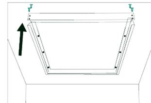
3. Once securely mounted to the ceiling disassemble one end (without mounting screws to the ceiling).
