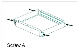
1. Assemble the four sides with 2 X screw A each to create the frame.
