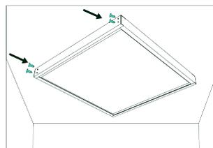
5. Reassemble the remaining end with screw A.
