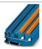
Feed-through terminal block, Connection type: Quick connection, Spring-cage connection, Cross section: 0.5 mm² - 2.5 mm², AWG :20- 14, Width: 6.2 mm, Color: blue, Mounting: NS 35/7,5, NS 35/15
