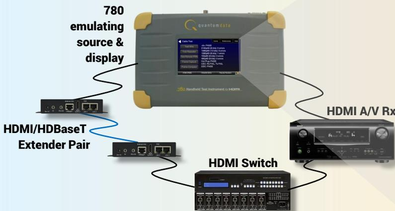
Example Network Test Setup
