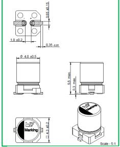
Example new drawings with direct dimensioning
