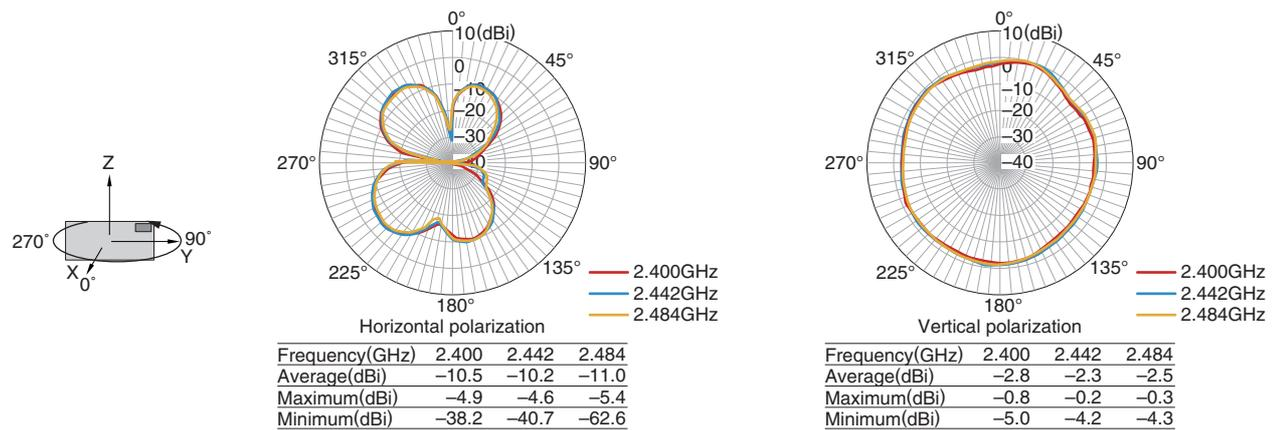
• Tested antenna has been soldered. Evaluation board size is 130x75x1 mm.
