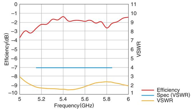
• Tested antenna has been soldered. Evaluation board size is 130x75x1 mm.
