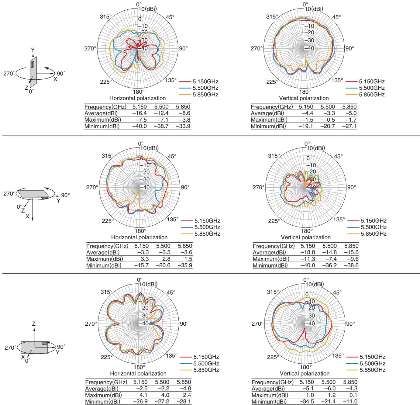
• Tested antenna has been soldered. Evaluation board size is 130x75x1 mm.
