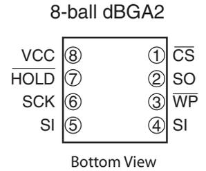
Block write protection is enabled by programming the status register with one of four blocks of write protection. Separate program enable and program disable instructions are provided for additional data protection. Hardware data protection is provided via the  $\overline{WP}$  pin to protect against inadvertent write attempts to the status register. The  $\overline{HOLD}$  pin may be used to suspend any serial communication without resetting the serial sequence.
