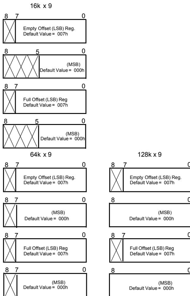
It is not necessary to write to all the offset registers at one time. A subset of the offset registers can be written; then by bringing the  $\overline{WEN2/LD}$  input HIGH, the FIFO is returned to normal read
