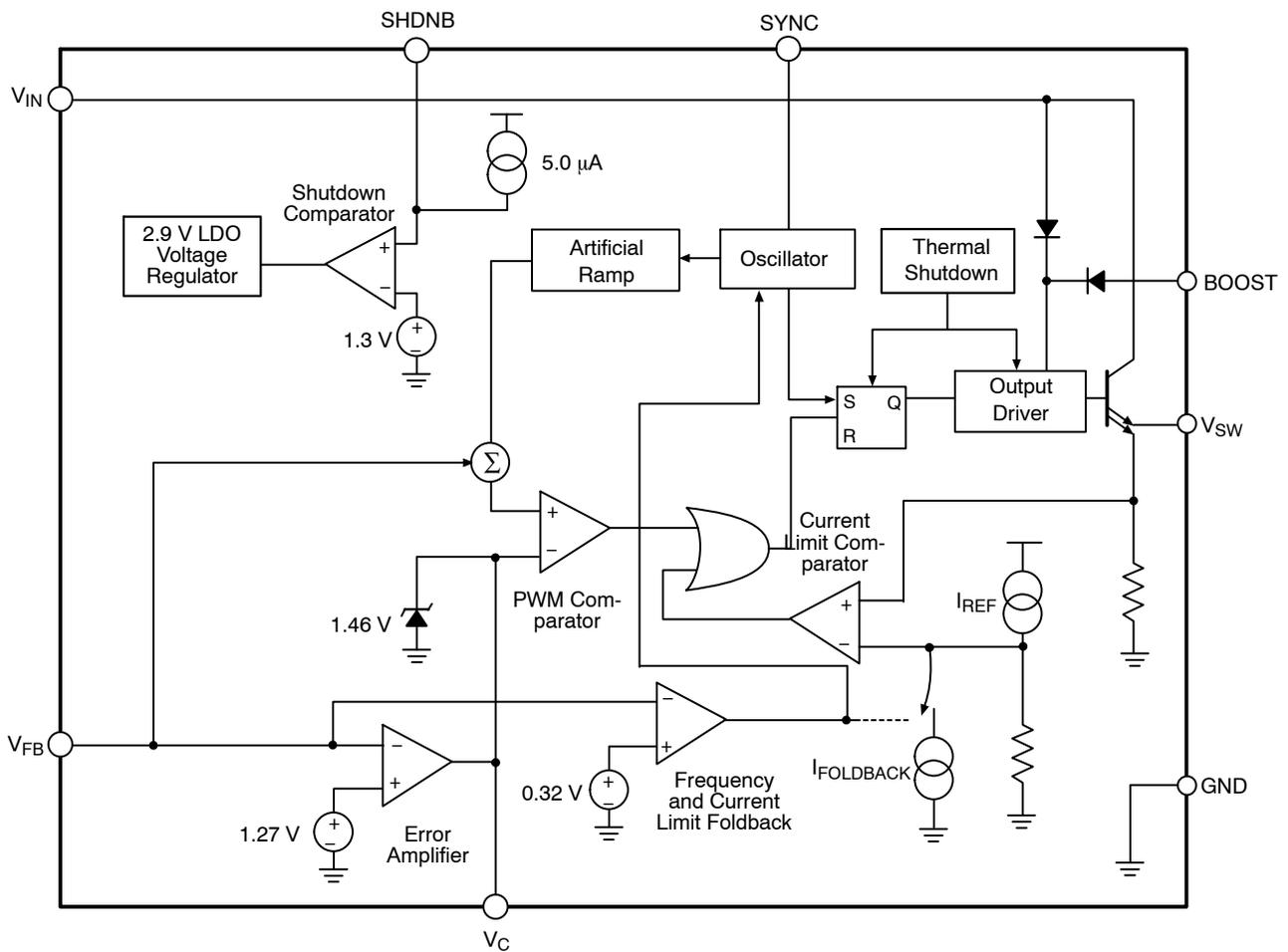
**Figure 2. Block Diagram**
