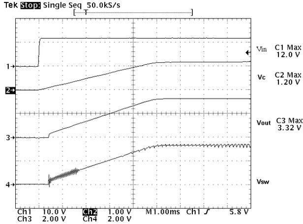
Figure 9. The Power Up Transition of NCV51411 Regulator
