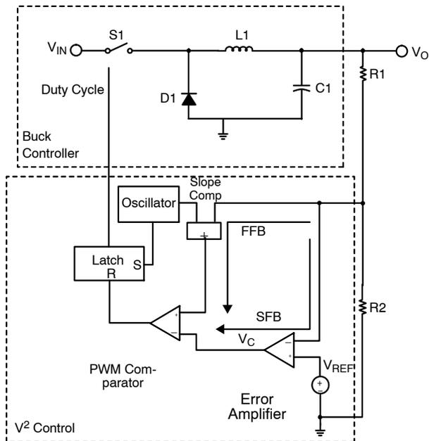
Figure 3. Buck Converter with V<sup>2</sup> Control.
