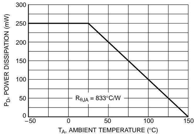
Figure 1. Derating Curve
