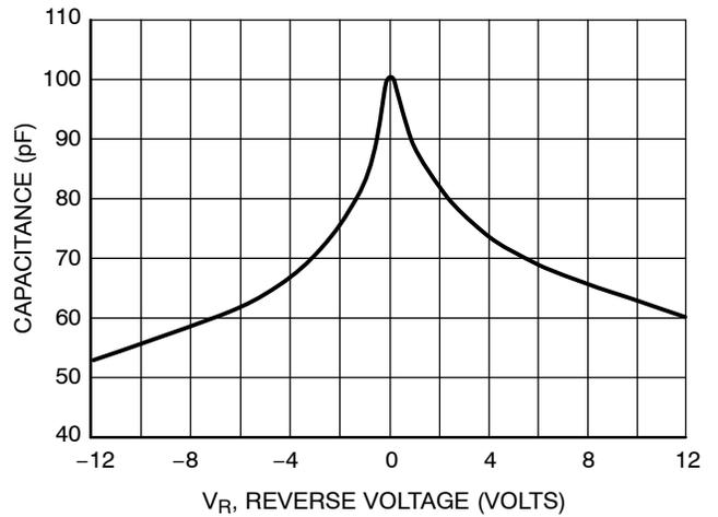
Figure 4. Typical Line Capacitance over Reverse Voltage
