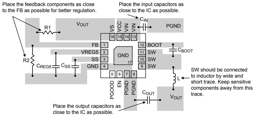
Figure 7. PCB Layout Guide
