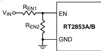
Figure 3. Resistor Divider for Lockout Threshold Setting
