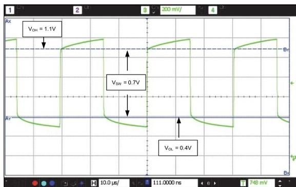
**Figure 4. SiT1532AI-J4-D14-32.768 Output Waveform (10 pF load)**
