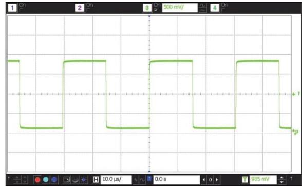
Figure 13. LVCMOS Output Waveform (V<sub>swing</sub> = 1.8V, SiT1532AI-J4-DCC-32.768)
