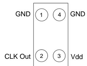
**Figure 1. Pin Assignments**
