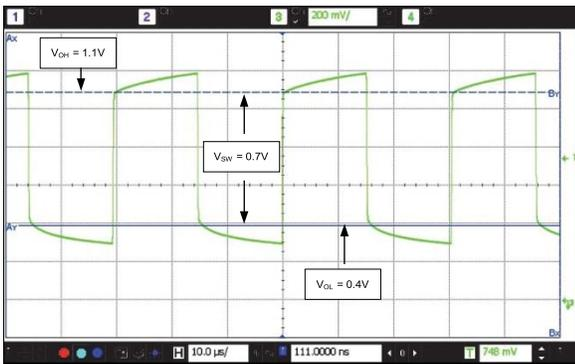
Figure 12. NanoDrive™ Output Waveform (V<sub>OH</sub> = 1.1V, V<sub>OL</sub> = 0.4V; SiT1532AI-J4-D14-32.768)
