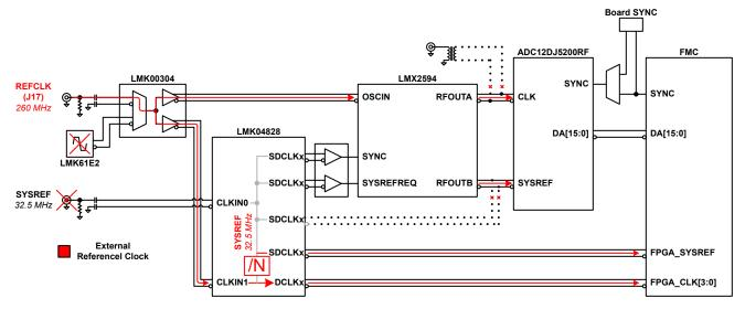
Figure 7-3. External Reference Clocking System Block Diagram
