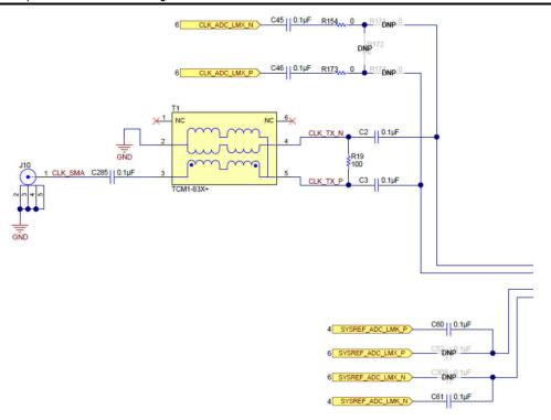
Figure 7-4. External Clock Configuration
