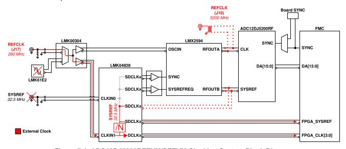
Figure 7-1. ADC12DJ5200RFEVM/SEEVM Clocking System Block Diagram
