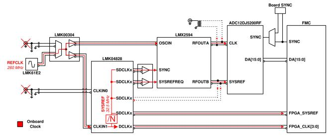
Figure 7-2. Onboard Clocking System Block Diagram
