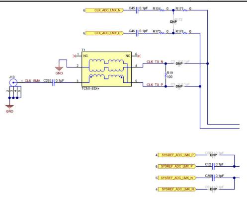
Figure 7-5. Onboard Clocking Configuration
