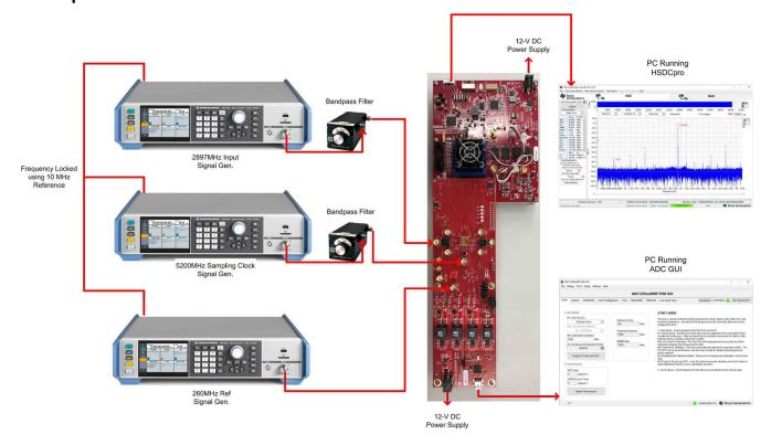
Figure 3-1. EVM Test Setup
