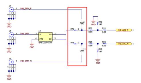
Figure A-1. Analog Input Path
