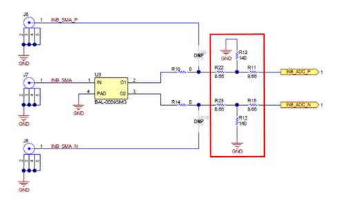
Figure A-2. 3 dB attenuation pad
