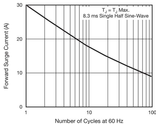
Fig. 2 - Maximum Non-Repetitive Peak Forward Surge Current
