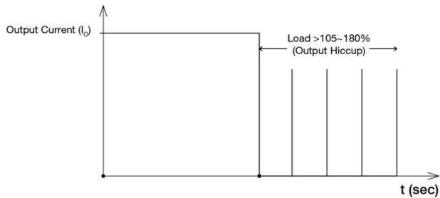
Additionally, if the  $I_o$  is <105-180% but >100% for a prolonged period of time (depending on the load), the Over Temperature Protection (OTP) will be activated due to high temperature on critical components. The power supply will then go into "Latch mode" until the PSU cools down and the AC power is recycled.
