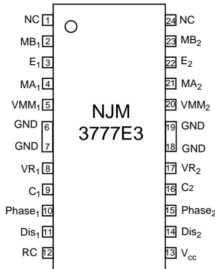
Figure 2. Pin configuration
