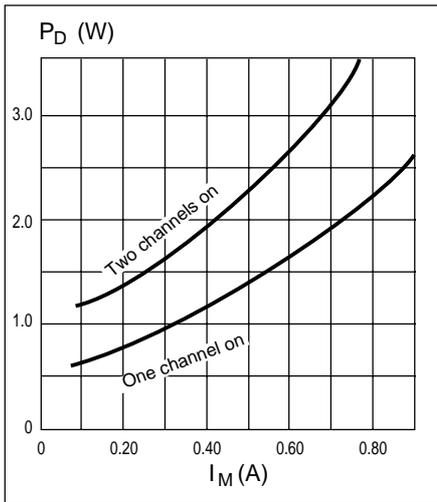
Figure 10. Power dissipation vs. motor current.  $T_a = 25^\circ\text{C}$
